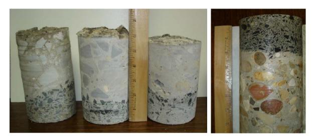
Figure 2. Cross Section of Two-Lift Section in Belknap Place, San Antonio (Ciggelakis et al. 2013; Taylor 2013).
