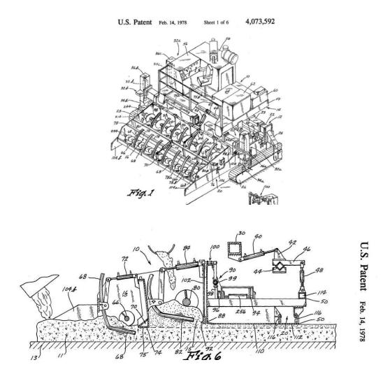
Figure 9. Gomaco GP-4000 Single Paver 2LCP System (Picture from Klein 2013).
