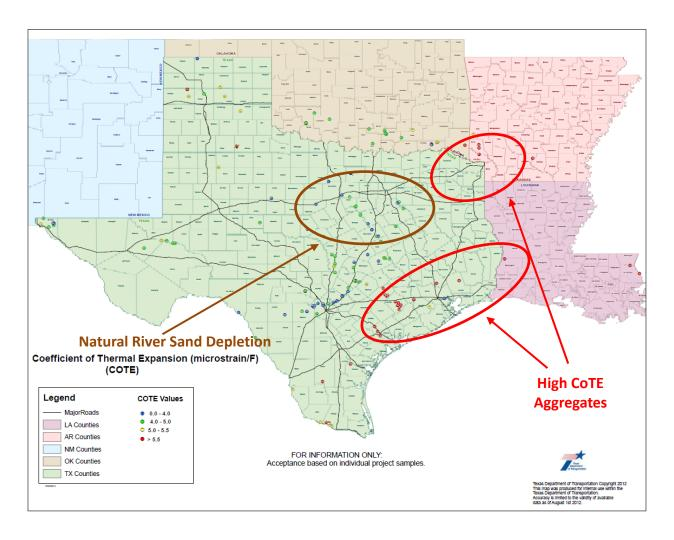
Figure 5. TxDOT Districts with Local Aggregates Not Appropriate for Conventional Concrete Paving.
