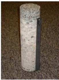
Figure 1. Typical 2LCP Construction and Pavement Cross Section (Photo Courtesy of Taylor [2013]).
