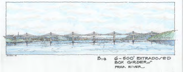
(b) B1-3–Six 500-Foot Extradosed Box Girders
