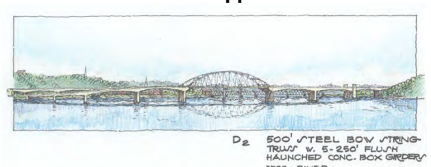
(f) D2–500-Foot Steel Bowstring Main Span with Five 250-Foot Haunched Concrete Girders
