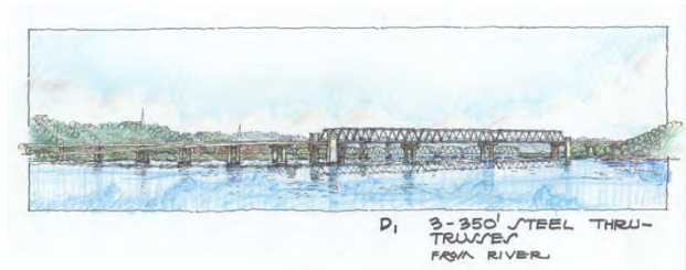
(e) D1–Three 350-Foot Steel Thru Trusses
