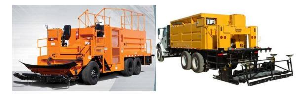
Figure 4-1. Self-Propelled Unit (Left) vs. Truck-Mounted Unit (Right).
