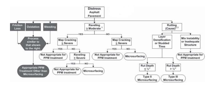
Figure 5-2. Conceptual Decision Tree for Asphalt Pavement Preservation and Maintenance Treatment Selection (21, 25)
