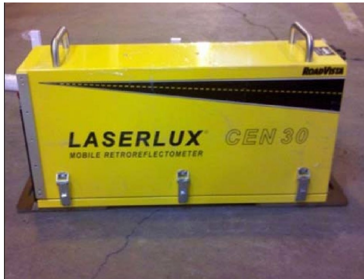
Figure 68 MnDOT LaserLux Outboard Unit
