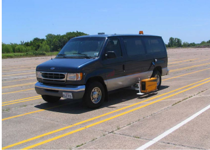
Figure 71 A Typical Pavement Marking Retro-reflectivity Measurement Device by FHWA
