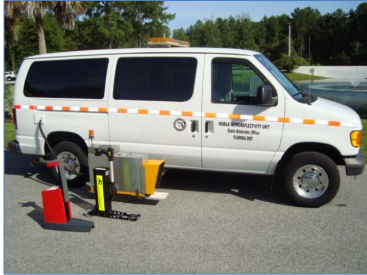
Figure 69 FDOT Test Instruments: Handheld Retro-reflectometers and Mobile Retro-reflectivity Unit (MRU)
