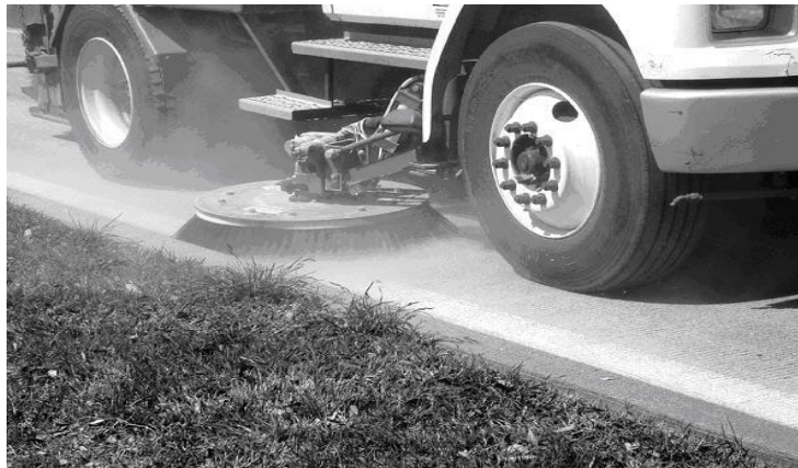
Figure 60 A Typical Broom Truck for Surface Preparations in Texas, New York, and Several Other States.
