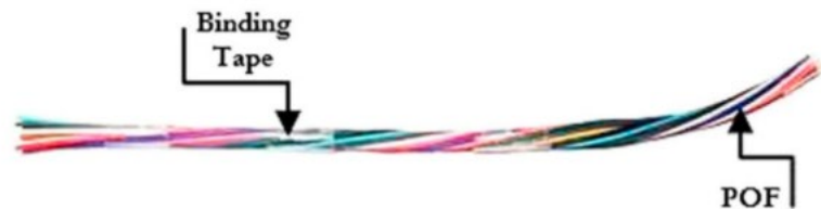
Figure 34 Optical Fiber Tendon (A)
