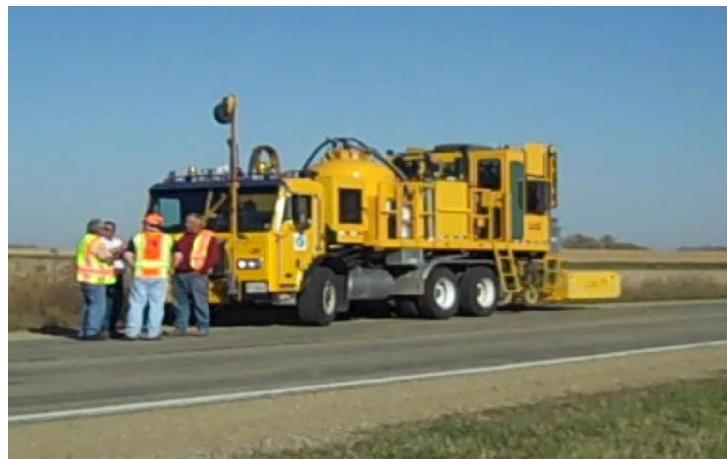
Figure 65 Water Based Striper Truck (MnDOT, 2015)
