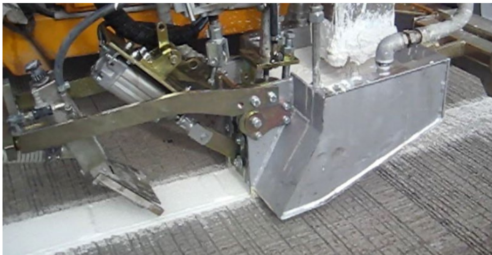
Figure 29 Rib Line Application Method
