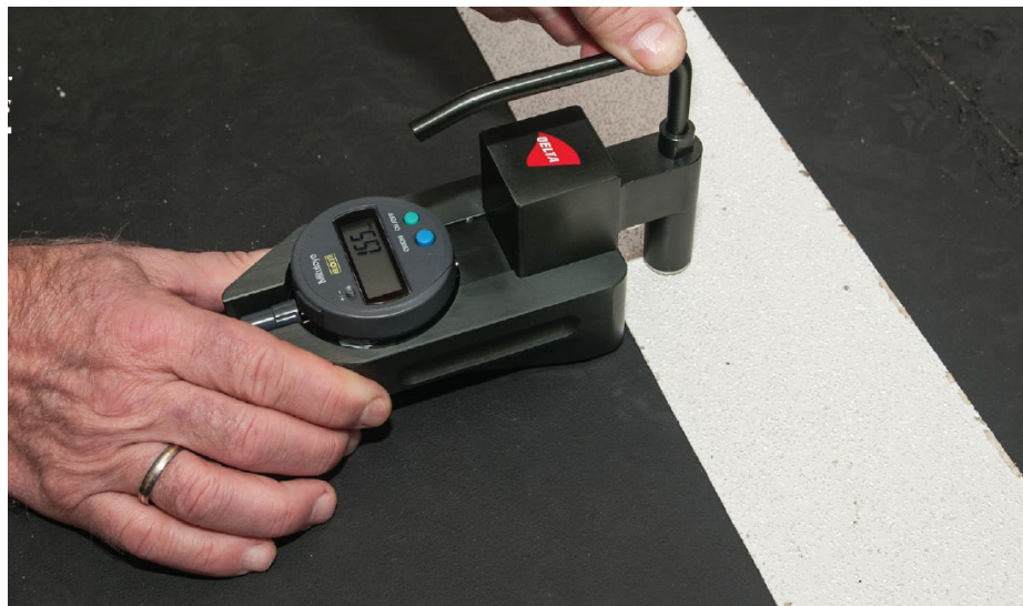
Figure 45 Marking Thickness Gauge (Delta and Forcetechnology, 2014)
