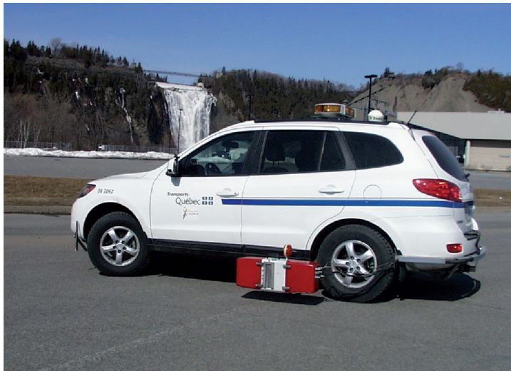
Figure 52 Mobile Retroreflectometer (Transports Quebec, 2019)
