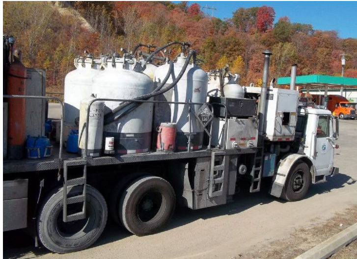
Figure 66 Epoxy Striper Truck (MnDOT, 2015)
