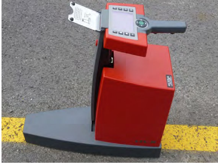
Figure 51 Hand-held Portable Retroreflectometer (Transports Quebec, 2019)
