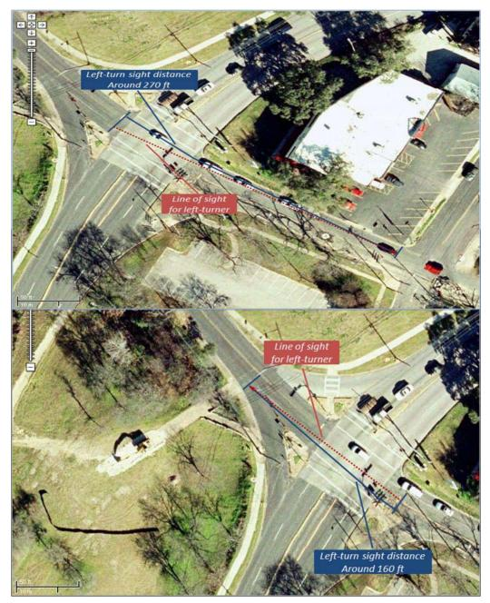
FIGURE 13. Sight Distances for the Left-Turn Movements at WB and EB Approaches of the Intersection at 29th St. & Lamar Blvd.
