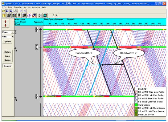
FIGURE 11. SYNCHRO Time-Space Diagram under Lead-Lead Phasing
