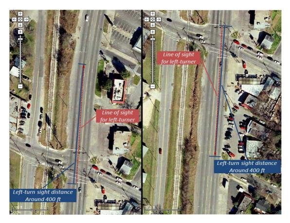
FIGURE 7. Sight Distances for the Left-Turn Movements at NB and SB Approaches of the Intersection at Airport Blvd. & 51st St
