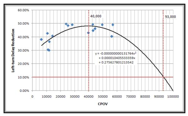
FIGURE 2. Plot of Left-Turn Delay Reduction versus Volume Cross Product for Two Opposing Lanes
