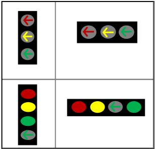
Figure 3 Recommended Left-Turn Signal Arrangement for PO Mode
