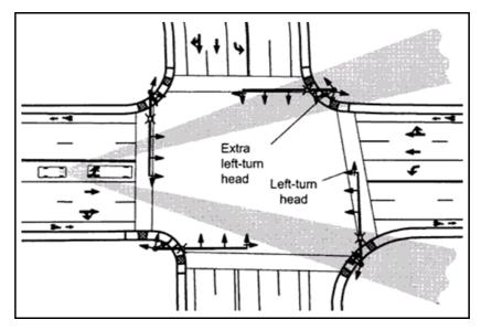
Figure 8 Far-Side Supplemental Left-Turn Signal Head Source: FHWA
