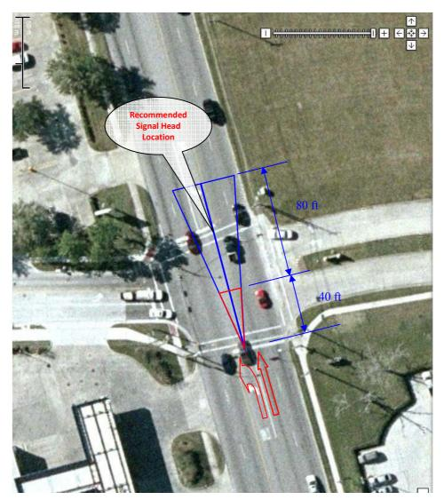
Figure 13 Recommended Signal Head Horizontal Location for Intersection at FM 518 & Calder Rd., League City, Texas.
