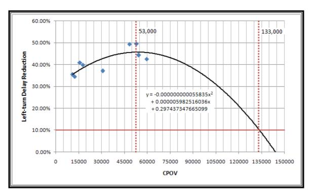
FIGURE 1. Plot of Left-Turn Delay Reduction versus Volume Cross Product for One Opposing Lane
