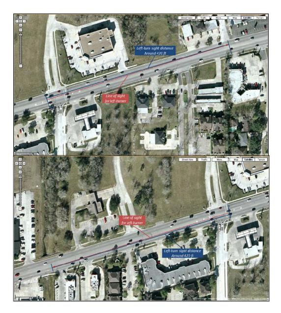
FIGURE 16. Sight Distances for the Left-Turn Movements at WB and EB Approaches of the Intersection at F.M. 518 & Calder Rd.
