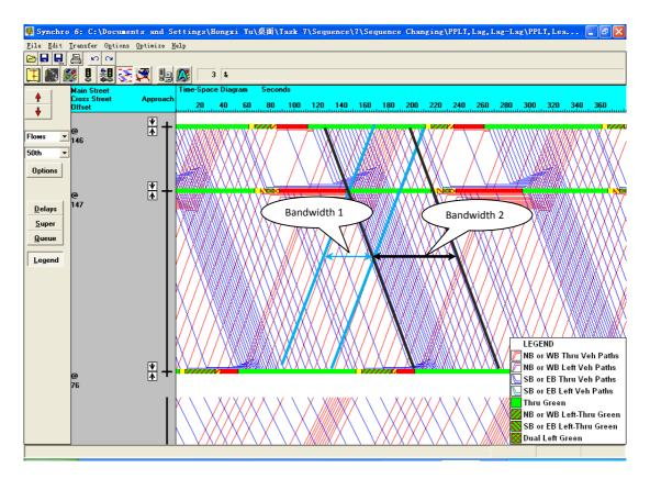
FIGURE 8. SYNCHRO Time-Space Diagram under Lag-Lag Phasing
