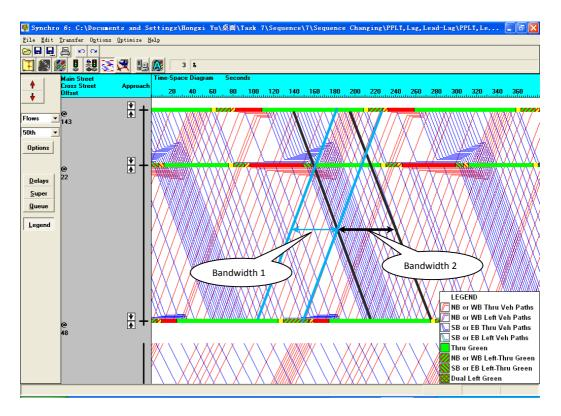
FIGURE 9. SYNCHRO Time-Space Diagram under Lead-Lag Phasing with NB Approach Having Leading Phase
