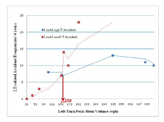
FIGURE 5. Left-Turn Accident Frequency versus Left-Turn Volume
