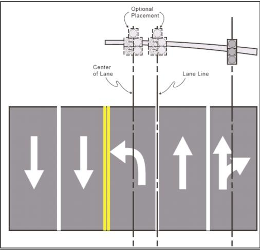
Figure 7 Overhead PPLT Display Placement Options Source: NCHRP Report 493
