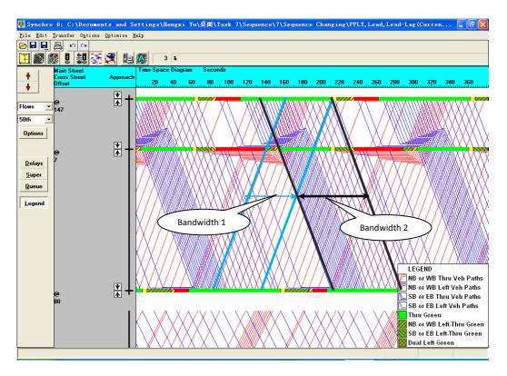
FIGURE 10. SYNCHRO Time-Space Diagram under Lead-Lag Phasing with NB Approach Having Leading Phase
