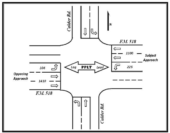
FIGURE 15. Basic Information for Intersection at F.M. 518 & Calder Rd.
