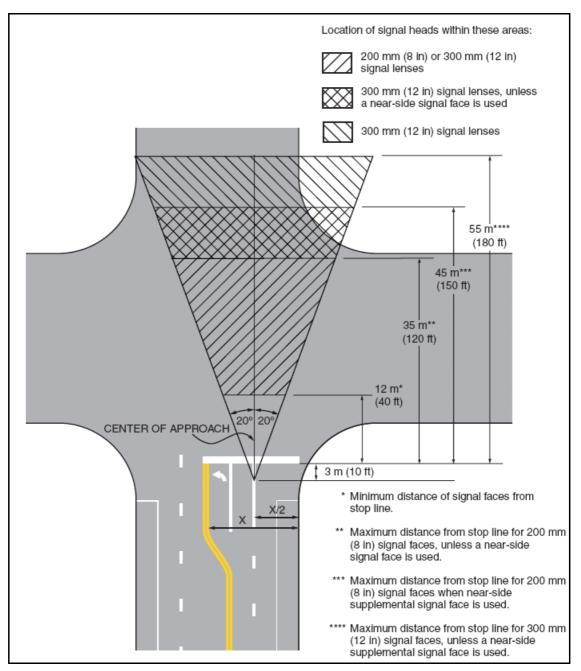
Figure 6 Criteria for Horizontal Location of Signal Face
