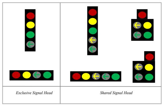
Figure 4 Recommended Left-Turn Signal Arrangement for PPLT Mode
