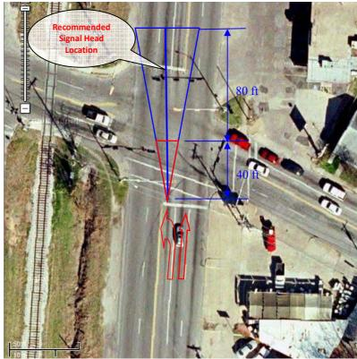
Figure 11 Recommended Signal Head Horizontal Location for Intersection at Airport Blvd. & 51st St. in Austin, Texas.
