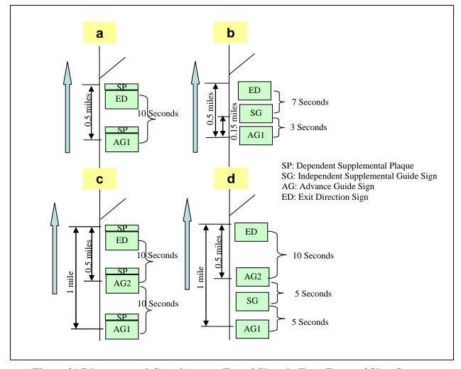
Figure 21 Distances and Gaps between Tested Signs in Four Types of Sign Groups
