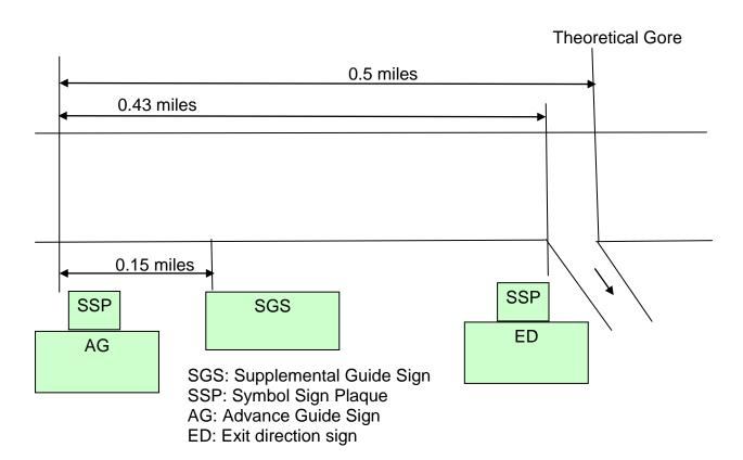
Figure 28 Placement of Different Types of Signs
