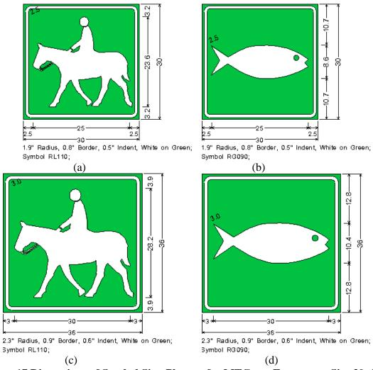
Figure 17 Dimensions of Symbol Sign Plaques for MTGs on Freeways—Size 30×30 Inches in (a) and (b), and Size 36×36 Inches in (c) and (d)—Plotted Using SignCAD
