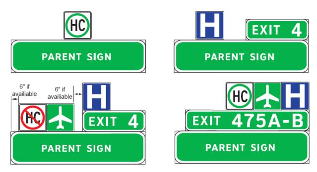
Figure 16 Overhead Freeway Guide Sign and Routing Plaque Typical Assemblies
