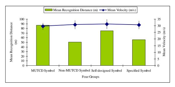
Figure 15 Mean Recognition Distance and Velocity for Test Symbol Groups
