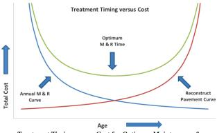
Treatment Timing versus Cost for Optimum Maintenance & Rehabilitation
