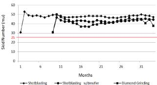
Comparison of Friction Treatments on Concrete Pavements
