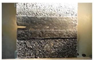
Example of Cohesion Failure
