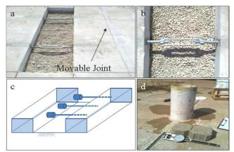
a) The movable joint system in the field b) The turn buckle used to move the slabs c) The schematic view of the movable joint system d) Flow test in the field
