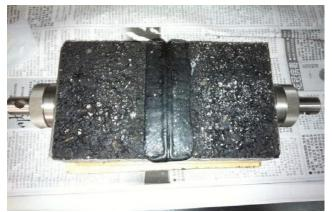
Seal Band Test Specimen
