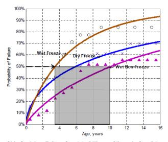
Chip Seal Age-Failure Graph in Different Climactic Conditions
