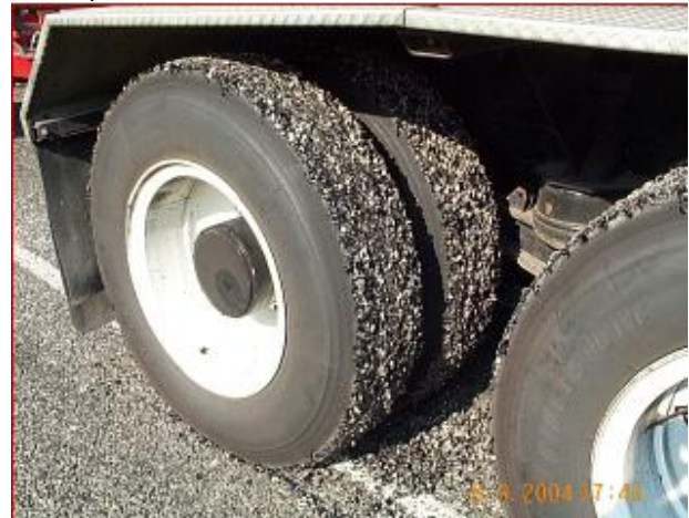
Figure 2. Seal Coat Damage due to SHL movement
