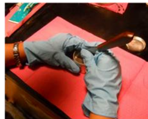
Cutting through the surface of the specimen to determine penetration depth
