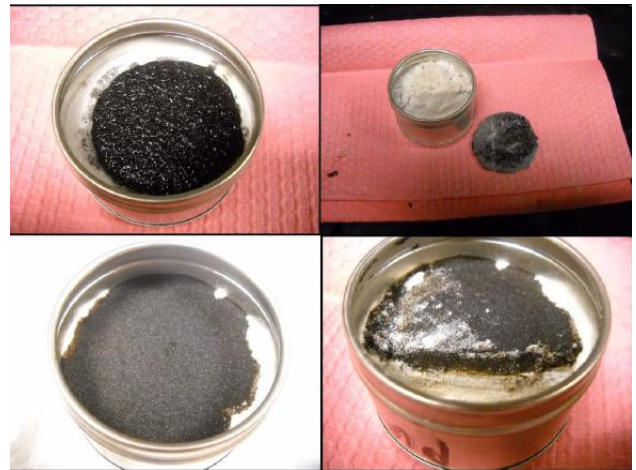
Figure 6- Penetration observed in emulsions (top) and cutbacks (bottom)
