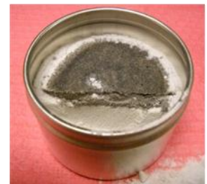
Figure 11 Penetration test for prime coat
