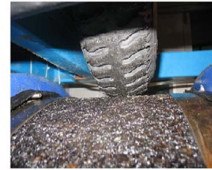
The Tire-Drive Pavement Function Accelerated Loading Test System (TRB 11-1997 pg. 3)
