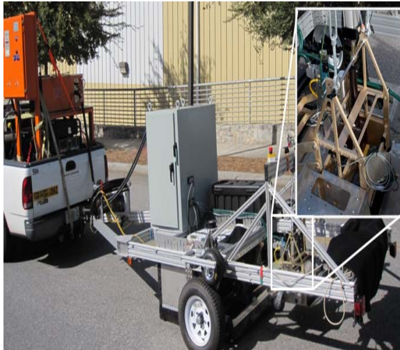
Picture of Prototype Crack Sealing Hardware with Detail of Applicators (TRB 11-1472 pg. 3)
