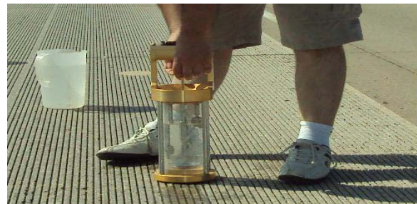
Outflow Meter Test Instrument (TRB 11-0346 pg. 6)
