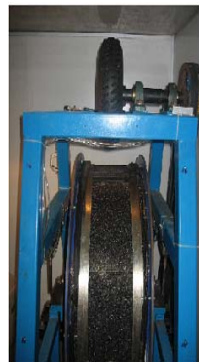
The Tire-Drive Pavement Function Accelerated Loading Test System (TRB 11-1997 pg. 3)
