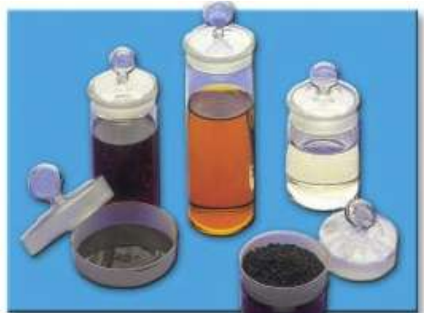
Separated Asphalt Components
