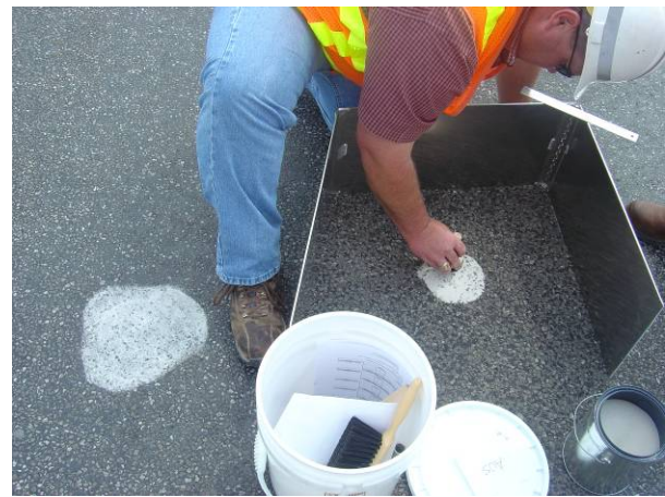
Figure 9. Performing the Sand Patch Test
