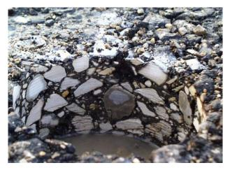
Aggregate breakdown during coring operation
