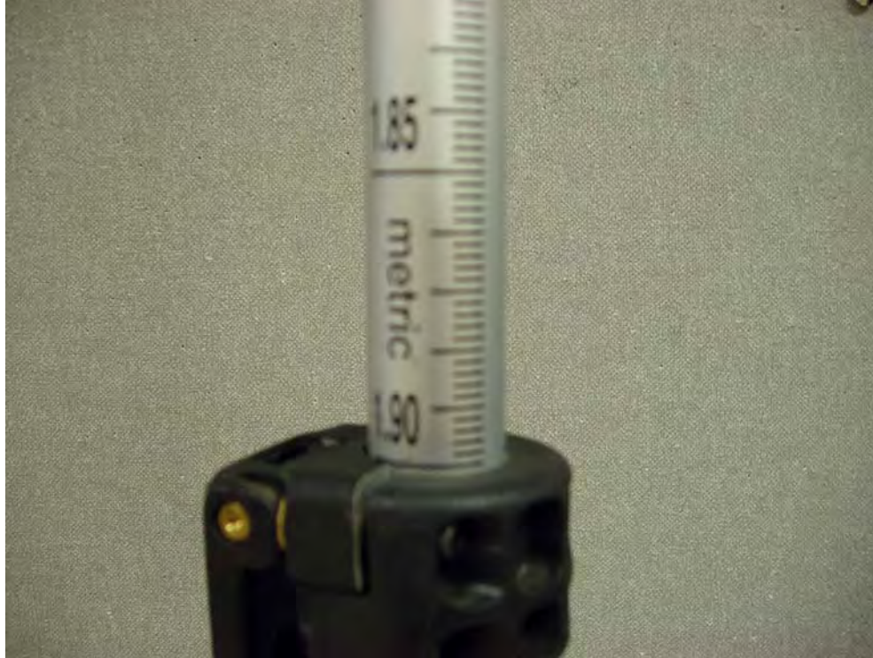
Figure 4.8 Surveyor's Rod Used for Deflection Measurements of September, 2002
