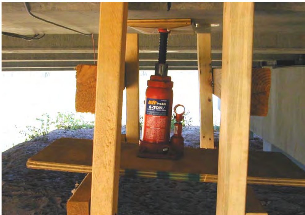
Figure 3.6 Jack System for Installing a Surface Strain Gauge on the Bottom of a Beam
