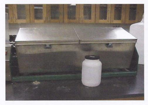
Figure 2: Extraction Vessel and Tumbler
