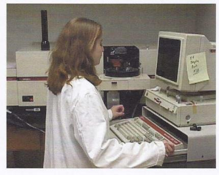
Figure 1. Graphite Furnace Atomic Absorption Spectrometer
