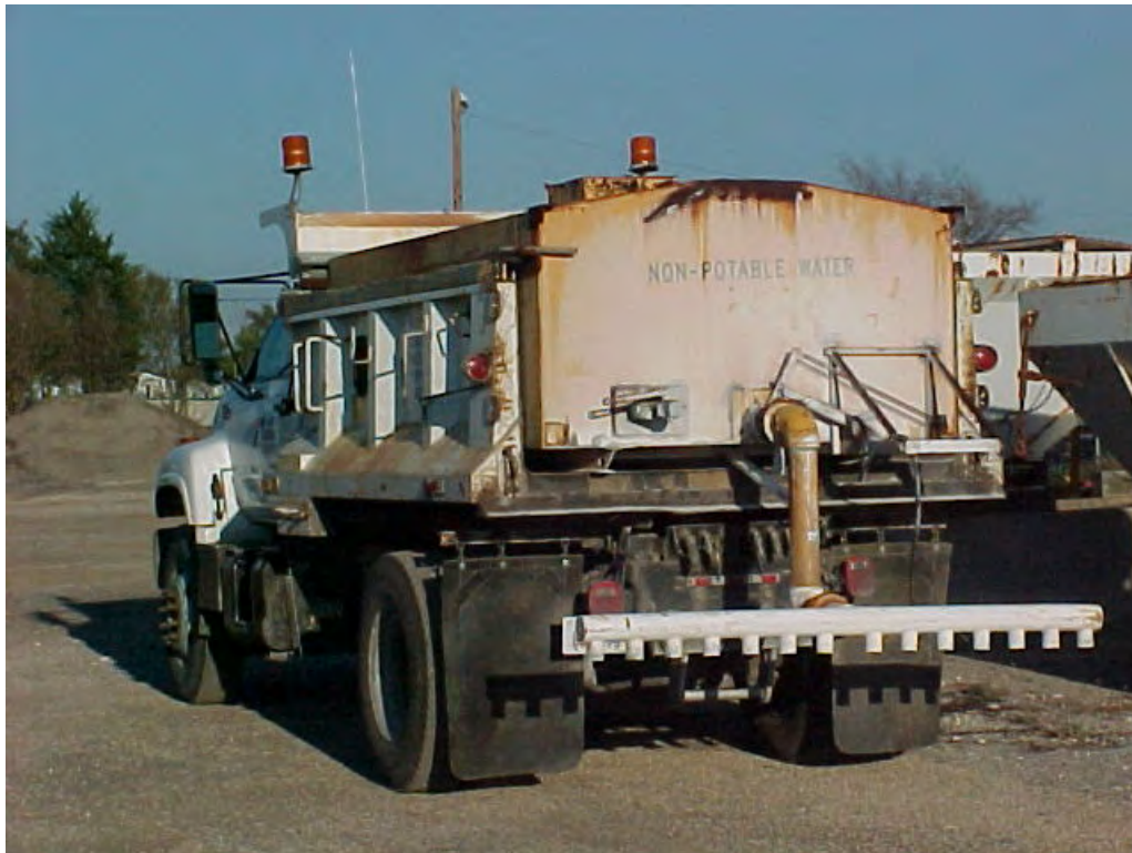
Figure 6.14 Application of Water Using a Standard Construction Water Truck
