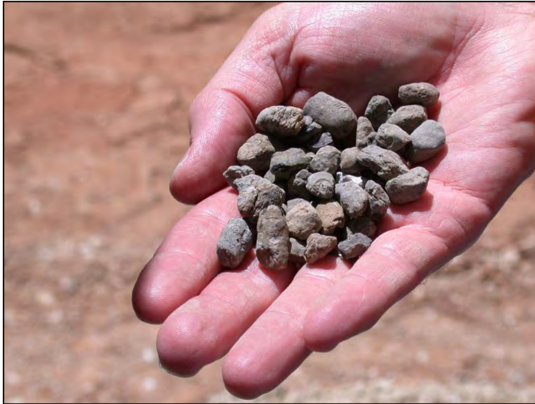
Figure 4.2 Dirty Seal Coat Aggregate
