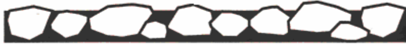
(b) Asphalt Binder Migrated to the Surface of Seal Coat Aggregate Causing Insufficient Voids Between Particles
