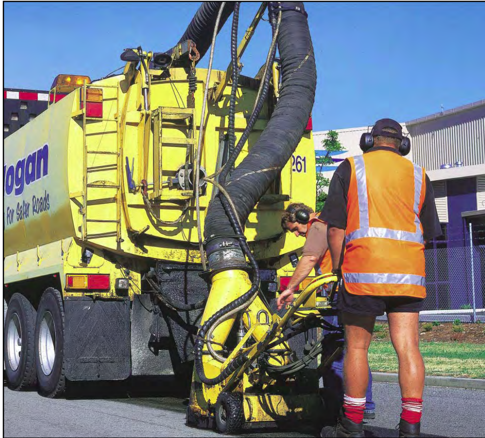
Figure 7.8 The UHP Watercutter Combines a Truck-Mounted UHP Pump, Water Supply, and Vacuum Recovery System with an Independently Operated Umbilical Deckblaster. Source: Fulton Hogan, Ltd. [ www.fh.co.nz ]
