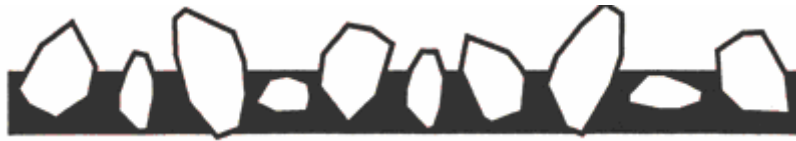
(a) Seal Coat Aggregate Particles Embedded in Asphalt Binder with Sufficient Voids Between Particles
