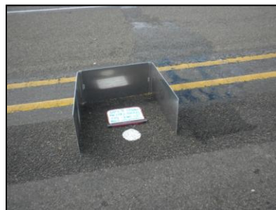
(a) wind screen set-up for sand patch
