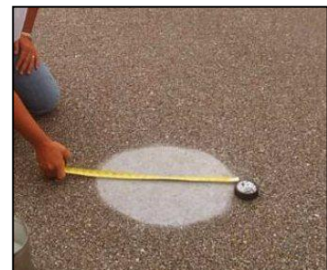
(c) measuring the sand patch
