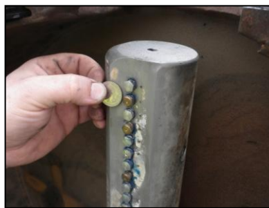
(b) water jet nozzles in the spray bar
