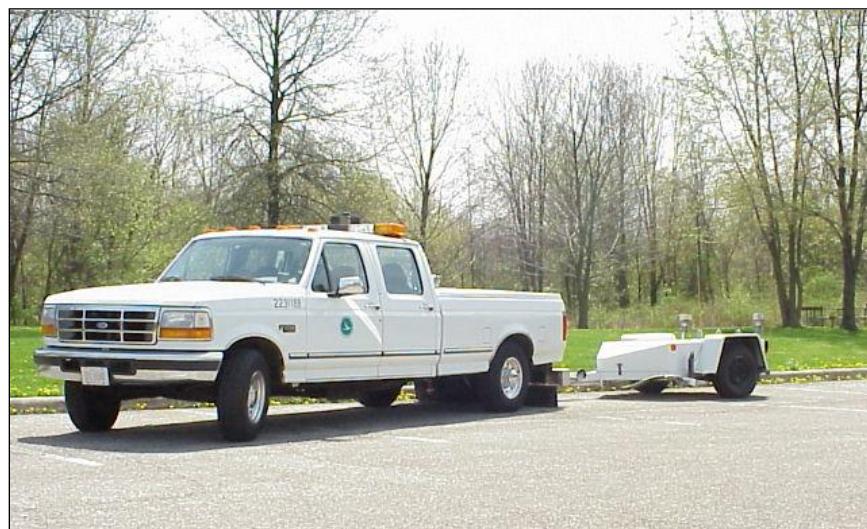
FIGURE 2.11. Skid truck used to measure Skid Number (SN) of pavement surfaces
