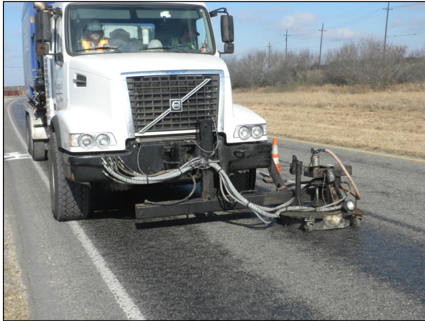
FIGURE 2.3. Cutting head, Rampart BlasterVac truck
