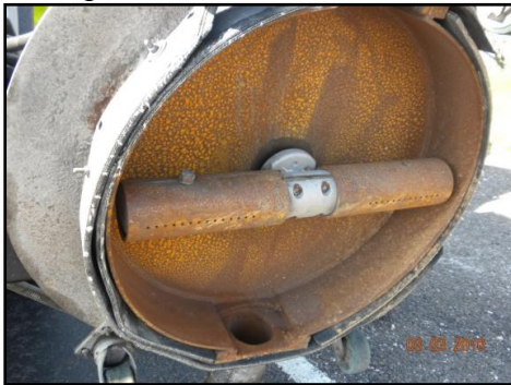
(e) UHP spray bar with nozzles
