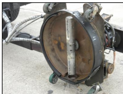
(a) cutting head with spray bar
