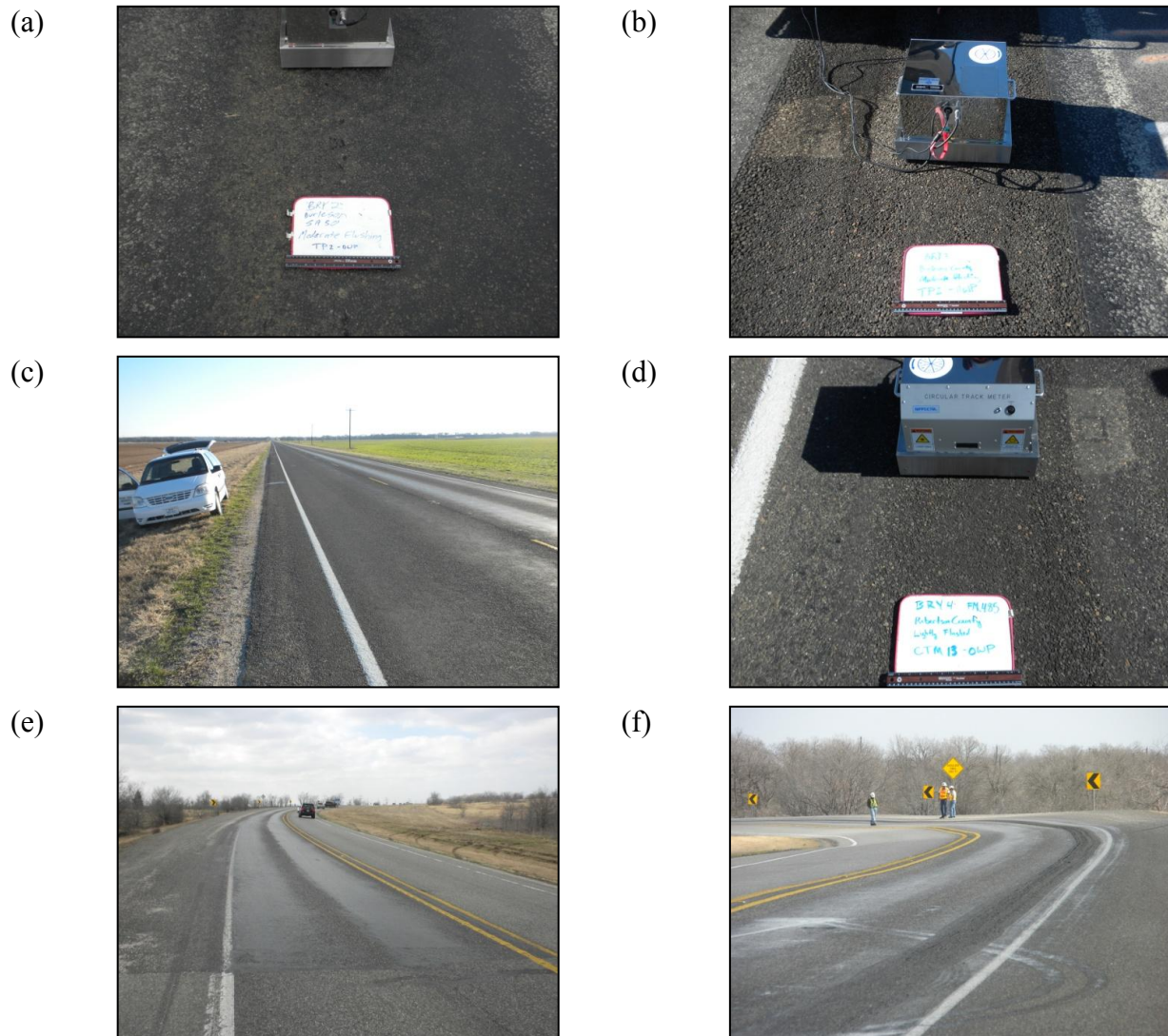
FIGURE 4.13. Test pavement pictures from Bryan District (a) BRY2 before treatment; (b) BRY2 soon after treatment; (c) BRY4 before treatment; (d) BRY4 soon after treatment; (e) BRY5 before treatment; (f) BRY5 soon after treatment
