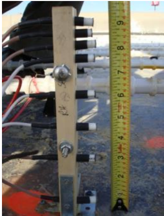
(a) Sensor for temperature and RH
