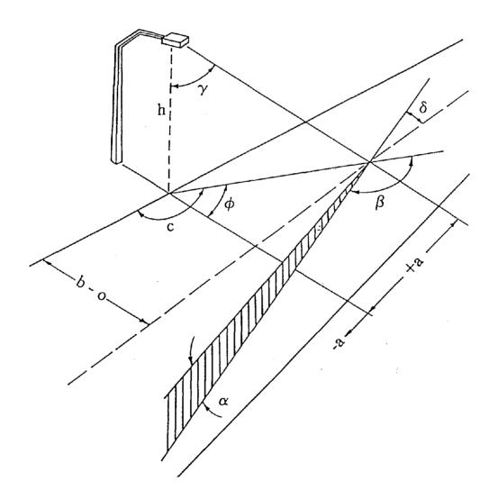
Figure 9. Schematic Diagram of Roadway Lighting
