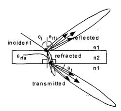
Figure 5. Reflection and Transmission Distributions
