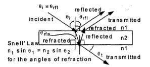
Figure 1. Specular Ray Tracing Model
