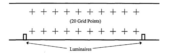
Figure 10. Network of Grid Points Between Luminaires Used to Calculate STV
