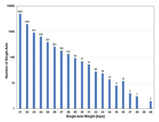
Figure 3.5 Illegal overweight single axle loading
