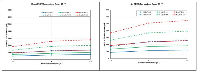
**Figure 6.8** Effect of longitudinal reinforcement depth on concrete vertical tensile stress at transverse crack area around the reinforcement for 11-in CRCP for 40 °F and 60 °F temperature drops
