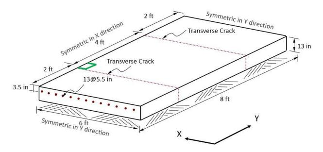
Figure 4.8 Geometry of model of LTE evaluation
