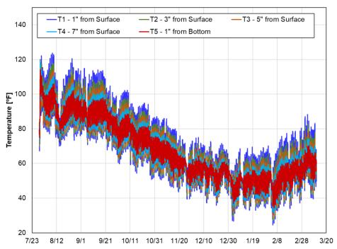
Figure 5.41 Pavement temperature profile in US62/180 El Paso test section
