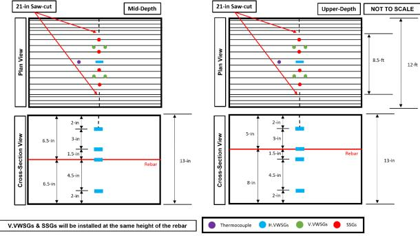
Figure 5.14 Plan view of typical gauge installation location in Hillsboro
