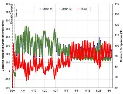
Figure 5.63 Longitudinal concrete strains at the mid-depth section in IH10 San Antonio
