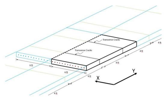
Figure 4.3 Geometry of symmetry model in ANSYS
