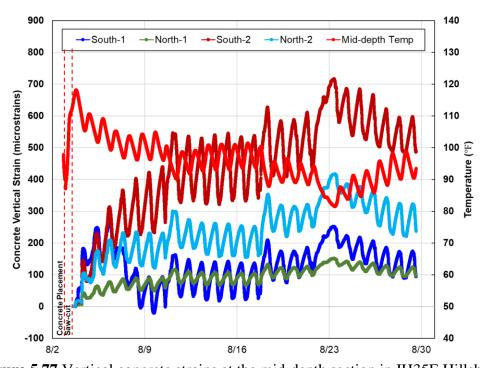
Figure 5.77 Vertical concrete strains at the mid-depth section in IH35E Hillsboro
