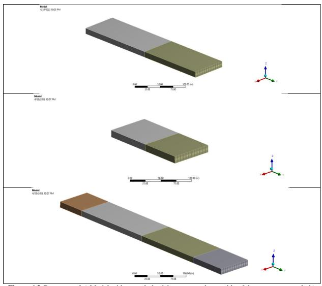
**Figure 6.3** Geometry of a) Model with one whole slab on east and west side of the transverse crack; b) Model with one half slab on east and west side of the transverse crack; c) Model with two slabs on east and two slabs on west side of the transverse crack
