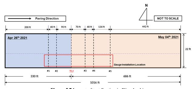
Figure 5.7 Layout of test Section in Waxahachie
