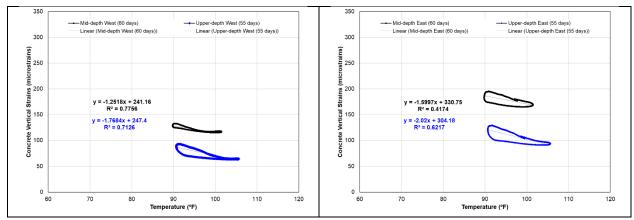
**Figure 5.68** Vertical concrete strains versus temperature of mid-depth and upper depth sections in IH10 San Antonio
