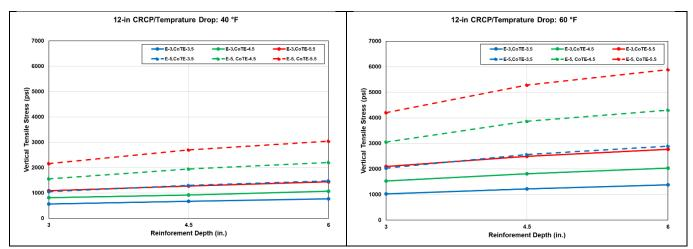
**Figure 6.9** Effect of longitudinal reinforcement depth on concrete vertical tensile stress at transverse crack area around the reinforcement for 12-in CRCP for 40 °F and 60 °F temperature drops
