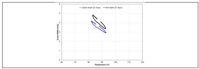
**Figure 5.76** Crack width versus temperature of mid-depth and upper depth sections in IH35E Hillsboro
