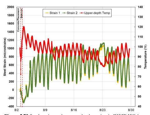
Figure 5.72 Steel strains at the upper-depth section in IH35E Hillsboro
