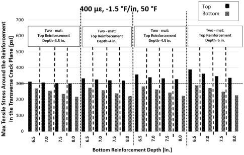
**Figure 4.33** Comparison of concrete stress on top surface between top and bottom reinforcement layer in two-mat design for 400 με ultimate drying shrinkage
