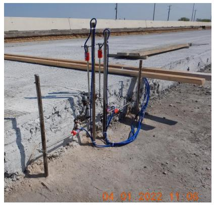
Figure 5.5 Typical Installation of Crackmeter in the field
