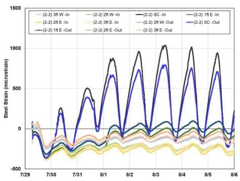
**Figure 5.27** Early-age steel strains at a distance from the sawcut in section 2-2 in US62/180 El Paso
