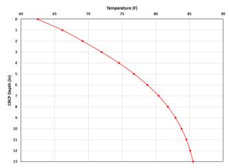
Figure 6.7 Temperature through the CRCP depth
