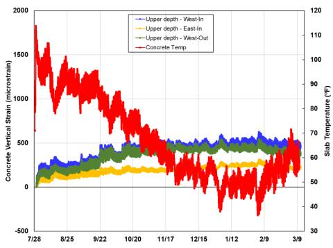
Figure 5.53 Long-term concrete vertical strains at the upper-depth section in US62/180 El Paso
