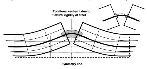
(b) Rotational restraint of steel on concrete subject to linear temperature gradient
