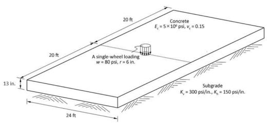
Figure 4.1 Geometric configuration of a concrete slab
