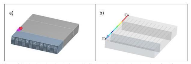
Figure 4.9 a) Loading location in the model, b) the path at loading location along the slabs
