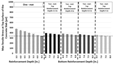
**Figure 4.29** Comparison of concrete vertical stress in one-mat and two-mat for 400 με ultimate drying shrinkage
