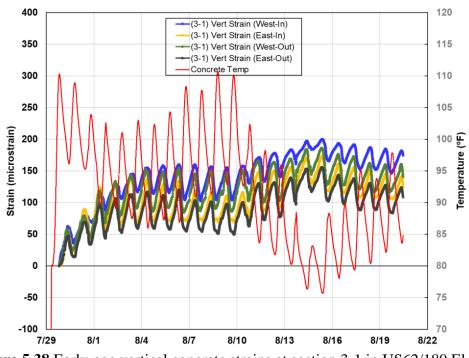
Figure 5.38 Early-age vertical concrete strains at section 3-1 in US62/180 El Paso
