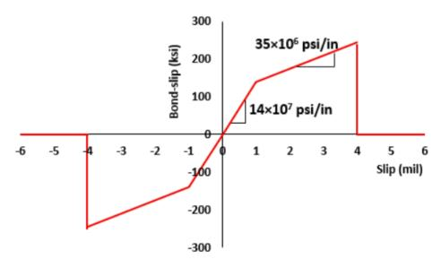
Figure 6.6 Bond-slip #2 behavior between concrete and longitudinal steel
