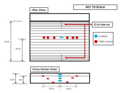
**Figure 5.15** Plan and cross-section views of typical gauge installation location at STA 212+00 in Hillsboro
