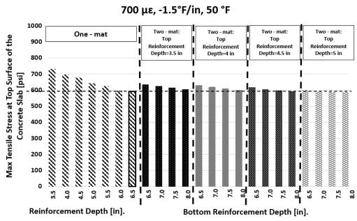
**Figure 4.30** Comparison of concrete vertical stress in one-mat and two-mat for 700 με ultimate drying shrinkage
