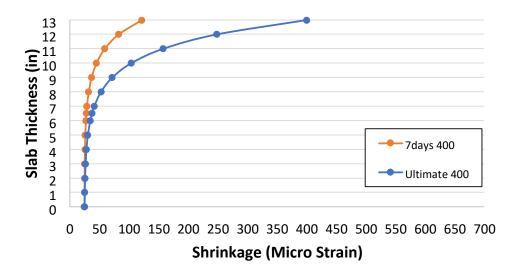
Figure 4.6 Shrinkage changes through the slab depth with ultimate value of 400 μ
