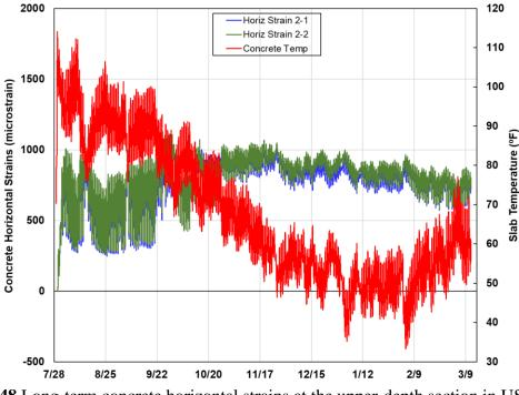
**Figure 5.48** Long-term concrete horizontal strains at the upper-depth section in US62/180 El Paso
