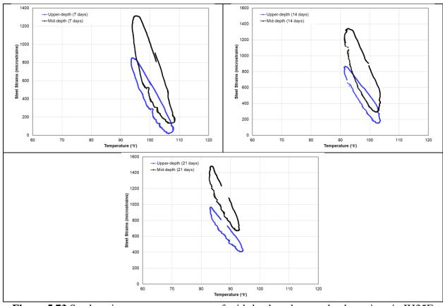
**Figure 5.73** Steel strains versus temperature of mid-depth and upper depth sections in IH35E Hillsboro
