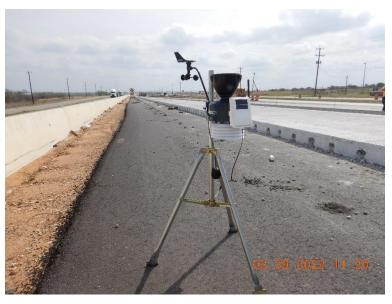
Figure 5.2 Davis Weather Station installed in field test site
