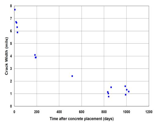
Figure 2.10 Variations of crack width over 3-yr time period
