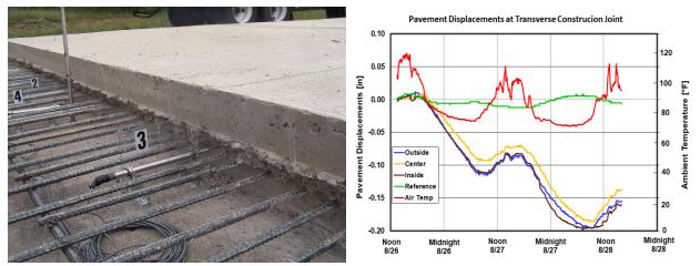
**Figure 2.12**-(a) Field instrumentation for slab movements at transverse construction joint (left); (b) Slab movements at transverse construction joint (right)
