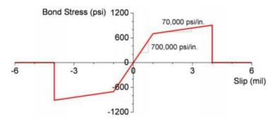
Figure 4.5 Bond-slip behavior between concrete and longitudinal steel
