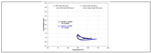
**Figure 5.65** Crack width versus temperature of mid-depth and upper depth sections in IH10 San Antonio
