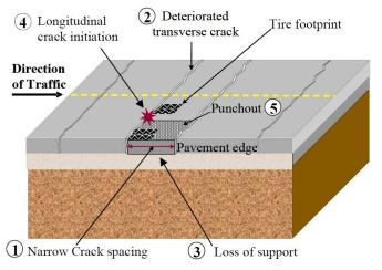
Figure 2.3 Punchout distress process adopted in MEPDG
