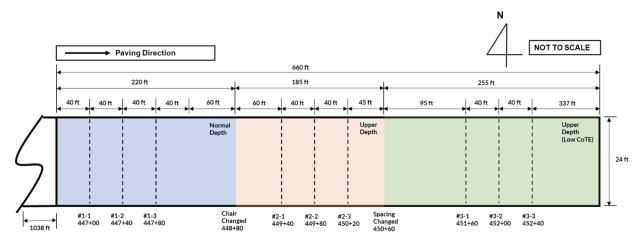
Figure 5.9 Layout of test Section in El Paso
