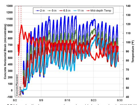
Figure 5.74 Longitudinal concrete strains at the mid-depth section in IH35E Hillsboro
