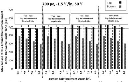
Figure 4.34 Comparison of concrete stress on top surface between top and bottom reinforcement layer in two-mat design for 700 με ultimate drying shrinkage
