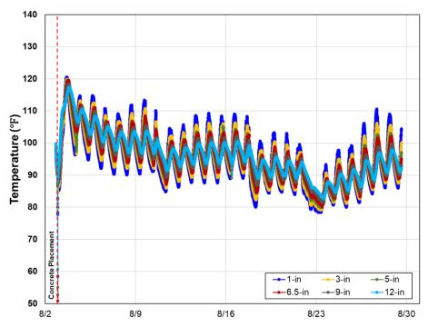
**Figure 5.69** Pavement temperature profile in IH35E Hillsboro test section
