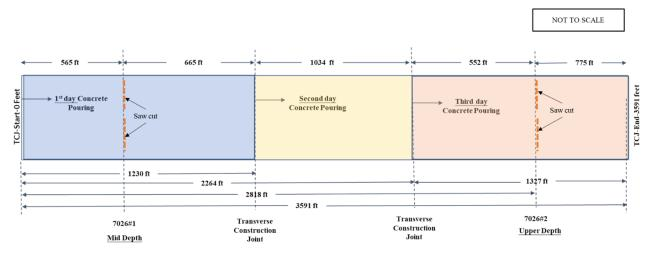
Figure 5.11 Layout of test Section in San Antonio
