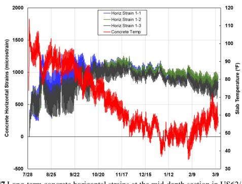
Figure 5.47 Long-term concrete horizontal strains at the mid-depth section in US62/180 El Paso
