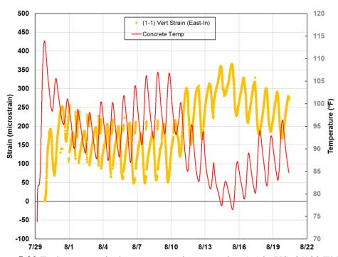
Figure 5.32 Early-age vertical concrete strains at section 1-1 in US62/180 El Paso
