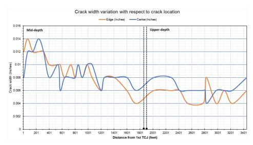
**Figure 5.94** Crack width measurement at the mid-depth and upper-depth sections in IH10 San Antonio
