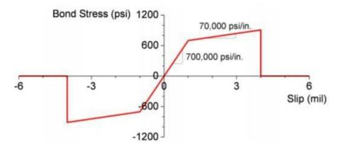
Figure 6.5 Bond-slip #1 behavior between concrete and longitudinal steel
