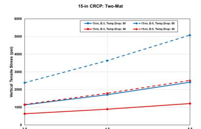
**Figure 6.12** Effect of longitudinal reinforcement depth on concrete vertical tensile stress at transverse crack area around the reinforcement for 15-in two-mat CRCP for 40 °F and 60 °F temperature drops
