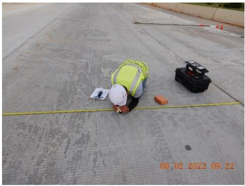
**Figure 5.93** Investigation of crack widths in mid-depth and upper depth section in IH10 San Antonio
