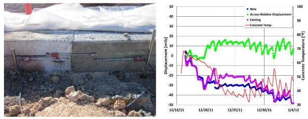
Figure 2.13-(a) Field instrumentation at a TCJ (left); (b) Slab displacements (right)
