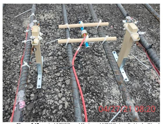
Figure 5.17 vertical VWSGs and Horizontal VWSGs installed in the Waxahachie
