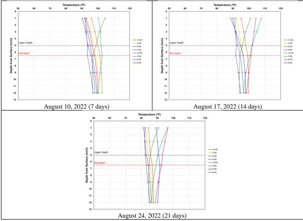
**Figure 5.70** IH35E Hillsboro test section temperature gradient at specific days from concrete placement
