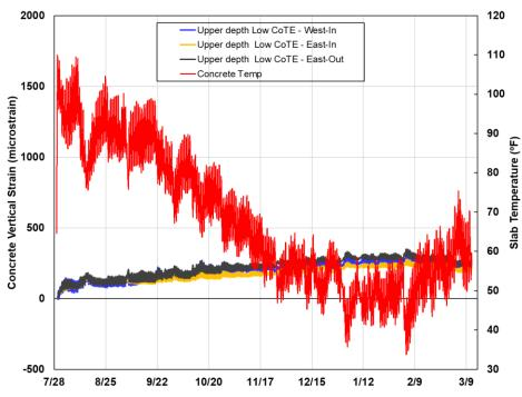
**Figure 5.54** Long-term concrete vertical strains at the upper-depth low CoTE section in US62/180 El Paso
