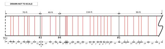
Figure 5.89 IH35 Waxahachie test section crack map at 257 days from concrete placement
