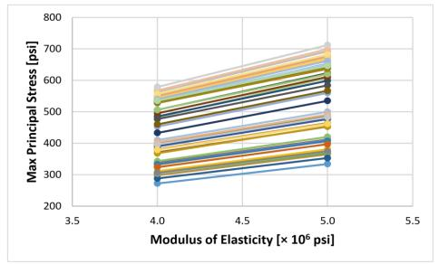
**Figure 4.17** Effect of modulus of elasticity on stress at transverse crack for 4-ft crack spacing and  $\alpha_c=3.5\times10^{-6}\ 1/^{\circ}F$
