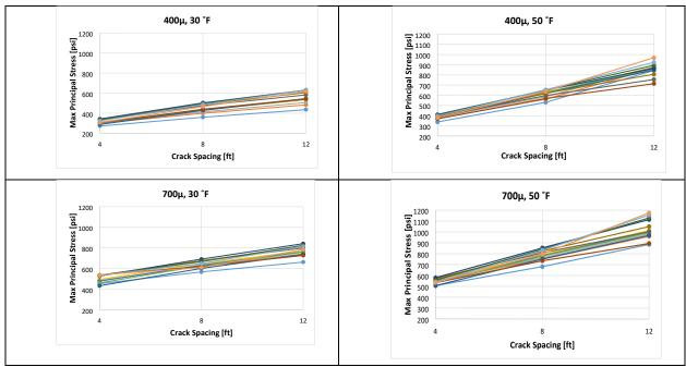
Figure 4.15 Effect of shrinkage on crack spacing
