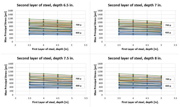
Figure 4.24 Effect of steel depth of first layer for 8-ft crack spacing
