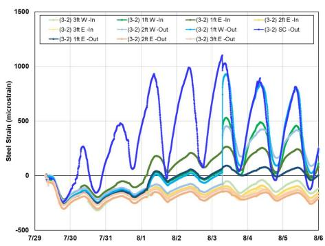
**Figure 5.28** Early-age steel strains at a distance from the sawcut in section 3-2 in US62/180 El Paso
