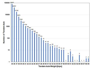
**Figure 3.6** Illegal overweight tandem axle loading
