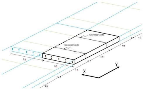
Figure 4.19 Geomtery of symmetry model in ANSYS for two-mat steel design
