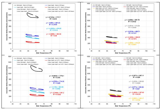
**Figure 5.55** Concrete vertical strains versus temperature of mid-depth, upper depth and upper depth low CoTE sections at 7, 28, 48, 78, 109, 139, 170, 201, and 224 days from concrete placement in US62/180 El Paso
