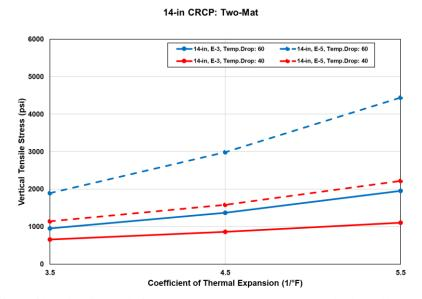
**Figure 6.11** Effect of longitudinal reinforcement depth on concrete vertical tensile stress at transverse crack area around the reinforcement for 14-in two-mat CRCP for 40 °F and 60 °F temperature drops
