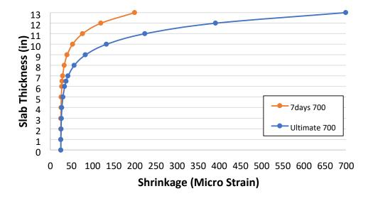
Figure 4.7 Shrinkage changes through the slab depth with ultimate value of 700 μ
