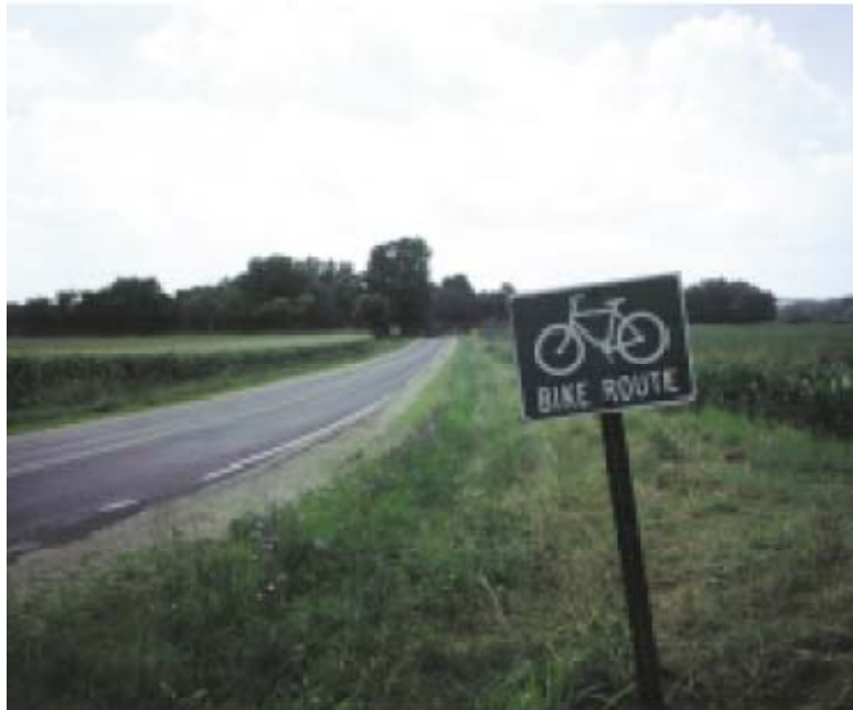
Figure 12: Signed Shared Roadway (Source: AASHTO, 1999)
