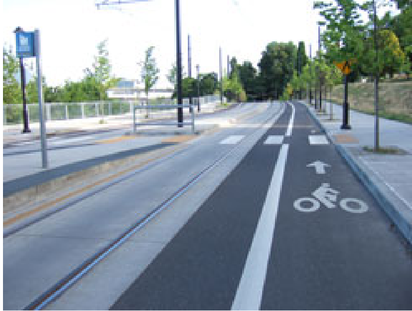
Figure 13: Bike Lanes (Source: PBIC, 2010)
