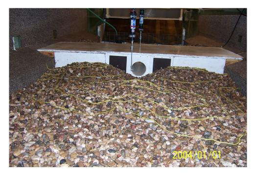
Figure 32: Photograph of Downstream Bedform Following Experiment on 2011/04/01, Experimental Model S-6-C
