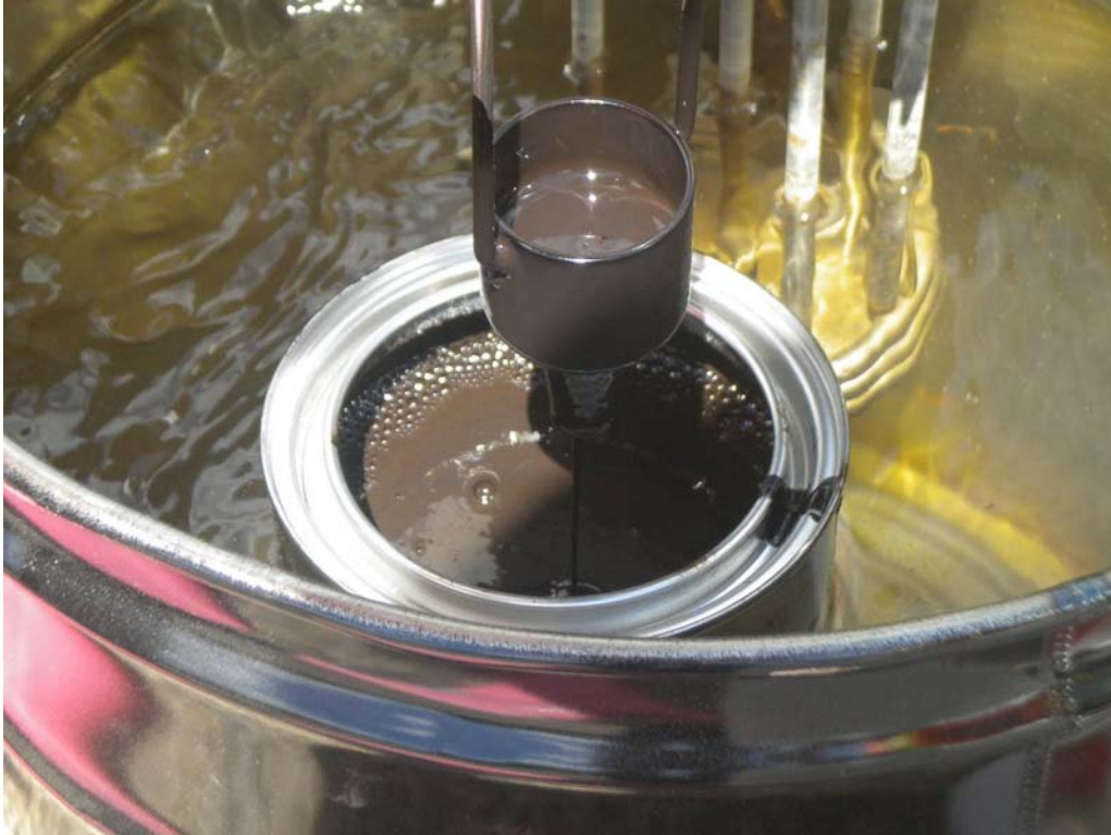
Figure 5.6 (b) Time Required for Emulsion to Drain from Shell Cup
