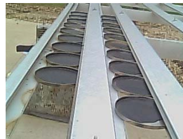
Measurement of Curing Rates Measured on TxDOT weathering racks
