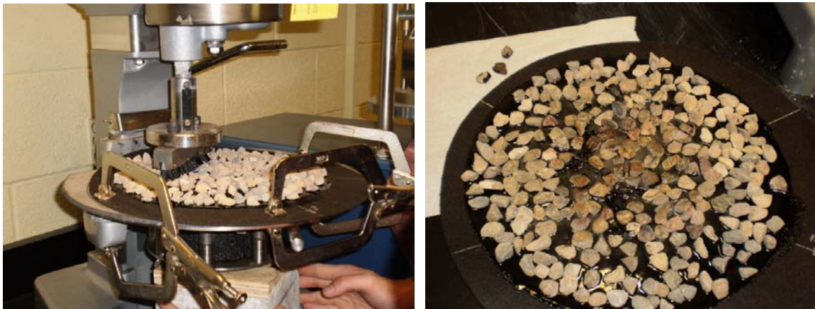
Figure 3.37 ASTM D7000 Sweep Test Apparatus and Test Specimen
