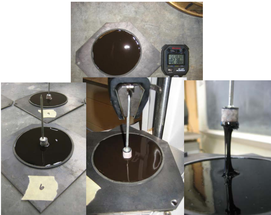
Figure 3.38. Images Depicting Different Stages of the Pull-Out Test
