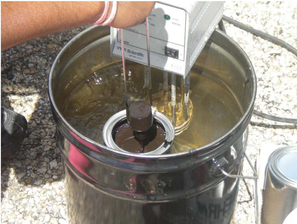
Figure 5.5 (a) Time Required for Emulsion to Drain from Shell Cup
