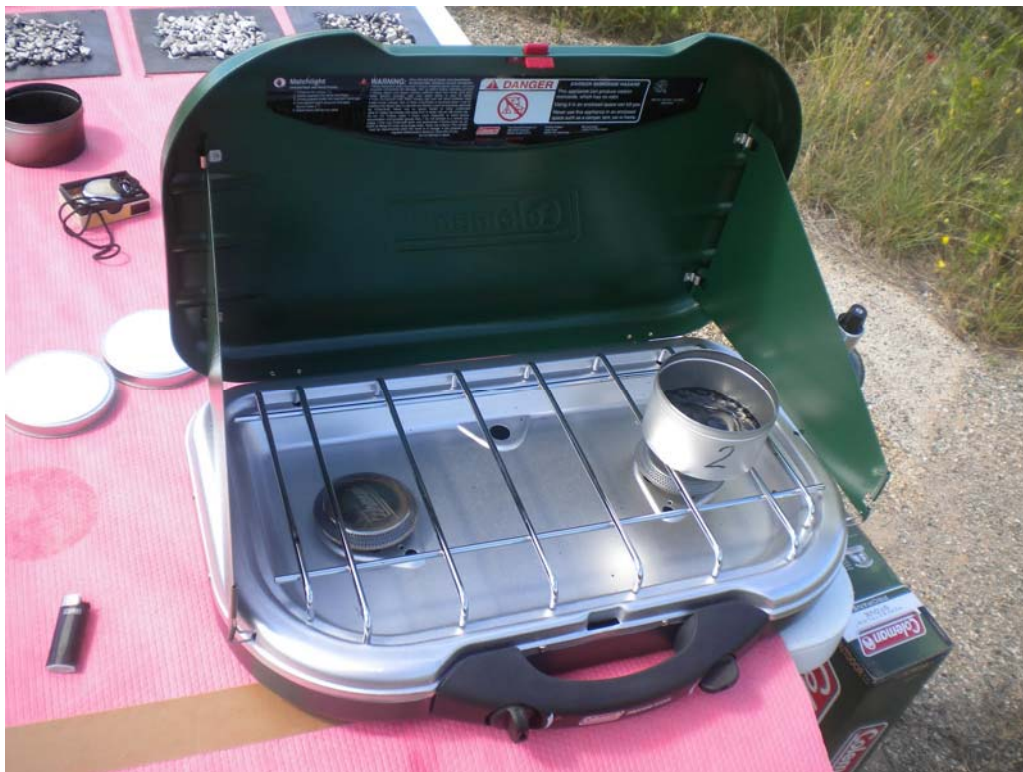
Figure 5.9 (a) Mass Loss Tests Carried Out in Field on Gas Oven
