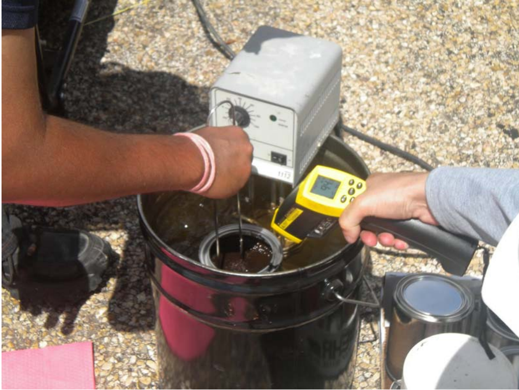
Figure 5.4 Infrared Temperature Gun to Record Temperature of Emulsion
