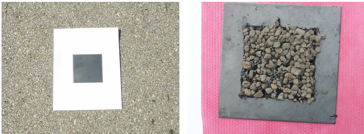
Figure 7.1 (a) Masked steel plates measuring 124mm × 124 mm (b) Final chip seal sample collected on the steel plate after 2 compaction cycles
