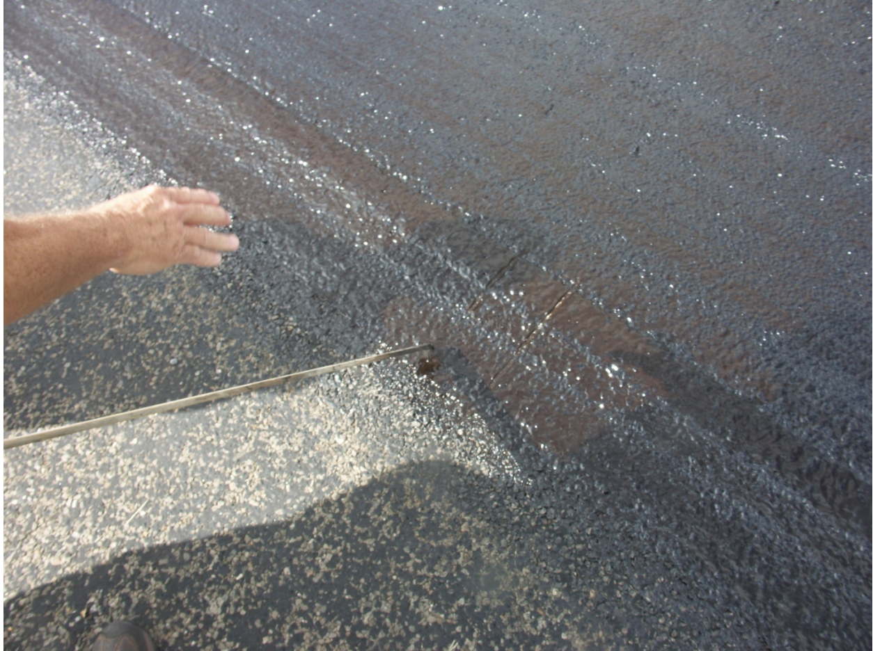
Figure 5.2 Demonstration of the “Stick Test” by the Field Inspector in Comanche, TX
