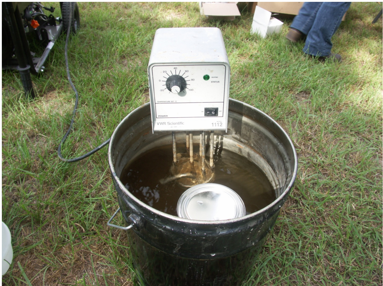
Figure 5.3 The Water Bath Used for Maintaining Steady Temperature of Emulsion Sample
