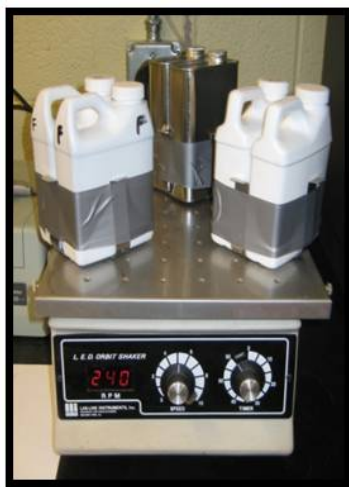
Figure 6.10 One-Pint Cans of Emulsion Mounted on Shaker Table to Simulate Transportation
