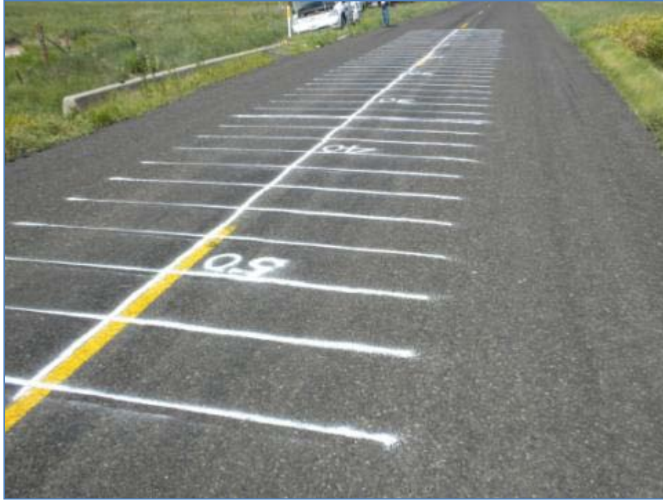
FIGURE 6.2. GAGE LINE CONSISTING OF TWO FOOT GRID MARKS TO DETERMINING TRUCK POSITIONS.
