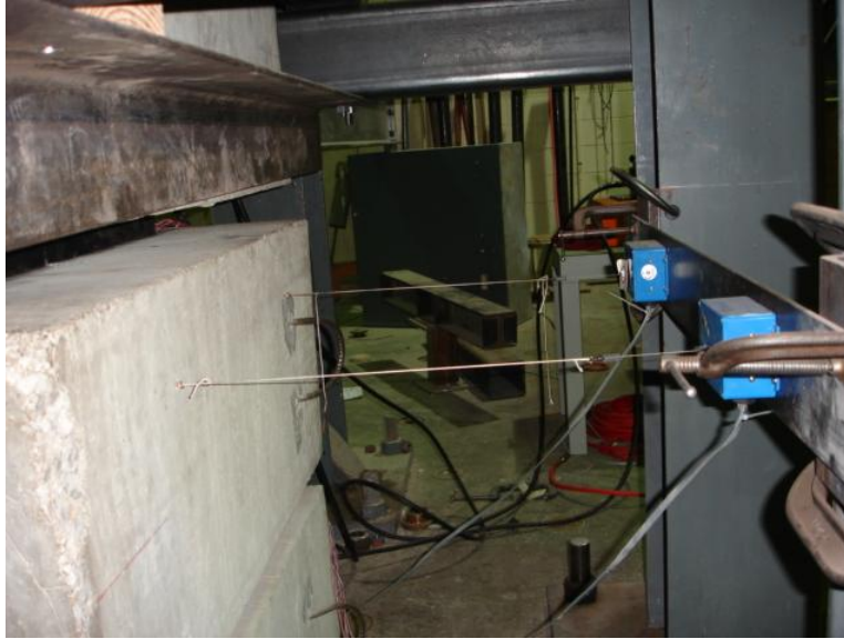
Figure 4.21 – Cable Extension Displacement Sensors – Longitudinal Direction
