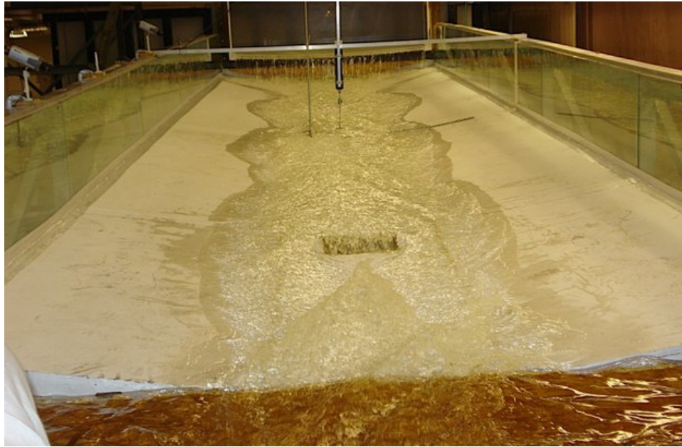
Figure 10: View of the system with an experiment in-progress. The image is looking upstream from the end of the flume. In the background the head tank and overflow weir is visible.
