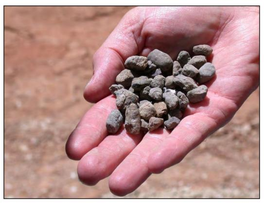
Figure 4.2 Dirty Seal Coat Aggregate
