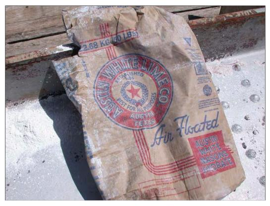
Figure 6.11 50-lb Bag, Type A Hydrated Lime
