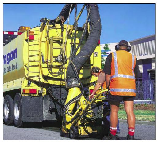
**Figure 7.8** The UHP Watercutter Combines a Truck-Mounted UHP Pump, Water Supply, and Vacuum Recovery System with an Independently Operated Umbilical Deckblaster.
