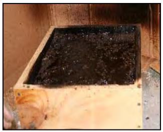
Figure 3.3 Prime Coated Specimen after Curing
