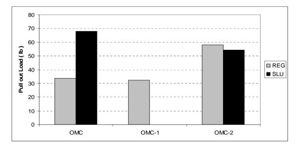
Figure 3.18 Pullout Strength for Four Base Moisture States and Two Surface Finishes
