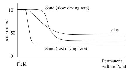
Figure 3.1 Typical Drying Curve for Sand and Clays (AE/PE vs Water Content)
