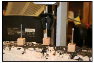
Figure 3.6 Pullout Strength Testing Arrangement
