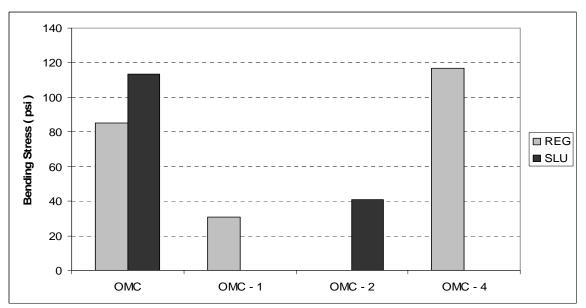
Figure 3.15 Flexural Strength for Four Base Moisture States and Two Surface Finishes
