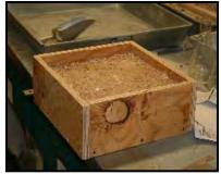
(a) Specimen mold (b) Compacted specimen Figure 3.2 Testing Mold and Prepared Specimen
