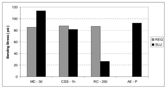
Figure 3.14 Flexural Strength of Primed Base for Four Binders and Two Surface Finishes
