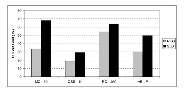
Figure 3.17 Pullout Strength of Primed Base for Four Binders and Two Surface Finishes
