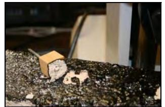
Figure 3.16 Unusual Failure in Pullout Test (See note in Table 3.6)
