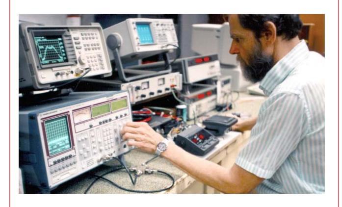
Figure 2: Bench-Top Testing with a TxDOT Radio in a Laboratory at Texas Tech University
