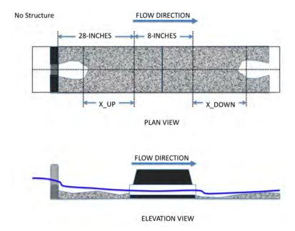
Figure 2.5: Sketch of Physical Model Experimental Configuration — No Structure Case.
