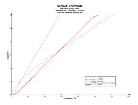
Figure A3 Graph of depth vs. discharge for the same conduit configurations.
