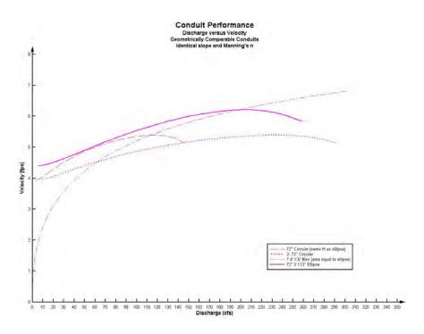
Figure A1 Graph of velocity vs. discharge for various conduit configurations.
