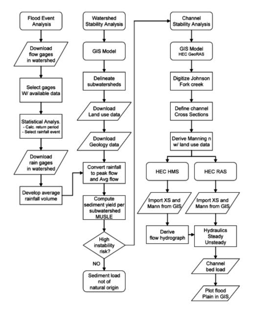
Figure 2.14: Flowchart of the analysis protocol used for the detailed numerical modeling developed by University of Houston researchers (Wang and Krou, 2008).
