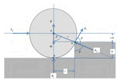
Figure 3.9: Sketch of sphere on flat bed with lateral motion restrained by a small step.
