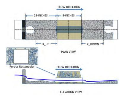
Figure 2.12: Sketch of Physical Model Experimental Configuration — Porous Culvert.
