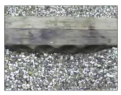
Figure 2.11: Image of Model Experimental Configuration — 4-Barrel Circular Culvert. Flow downstream is into the image.
