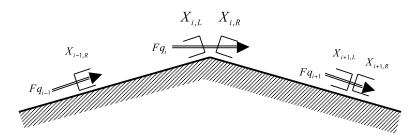
Figure 2.22: Schematic of bed flux through channel segments (Wang and Krou, 2008).
