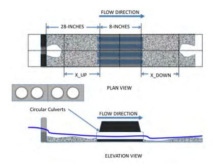
$\label{eq:configuration} \textbf{Figure 2.10: Sketch of Physical Model Experimental Configuration} \ -- \ 4\text{-Barrel Circular Culvert}.$
