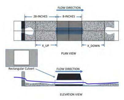
Figure 2.6: Sketch of Physical Model Experimental Configuration — Rectangular Culvert.
