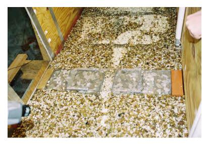
Figure 2.13: Image of Physical Model Experimental Configuration — Porous Culvert. Plastic cover representing roadbed in-place in this image.
