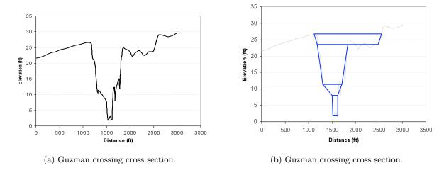
Figure 3.19: Johnson Fork Creek Guzman crossing surveyed and schematized cross sections.
