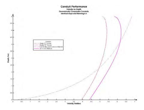
Figure A2 Graph of depth vs. velocity for the same conduit configurations.
