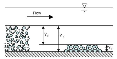
Figure 2.21: Schematic of the streambed armoring process (Wang and Krou, 2008).
