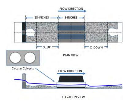
Figure 2.8: Sketch of Physical Model Experimental Configuration — 2-Barrel Circular Culvert.
