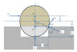
Figure 3.10: Geometry of sphere in a "pit." Flow is partially shielded by the pit.
