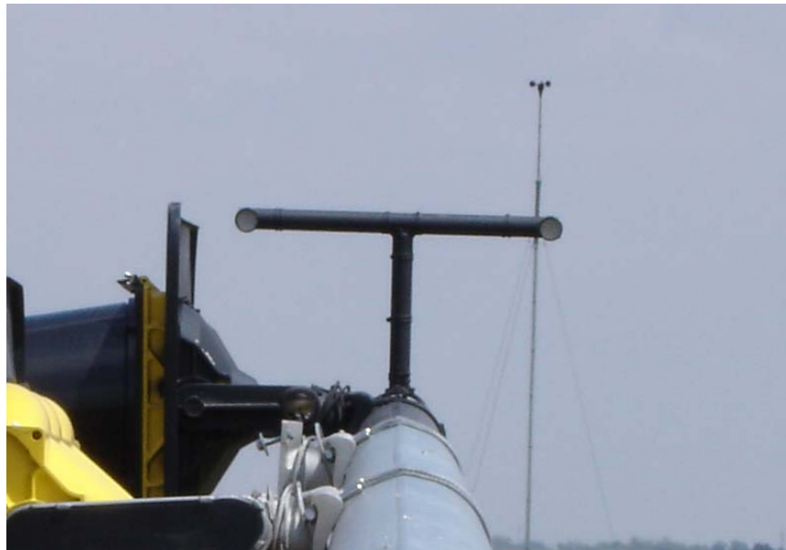
Figure 6. Infrared Target, As Viewed from the Top of the Pole
