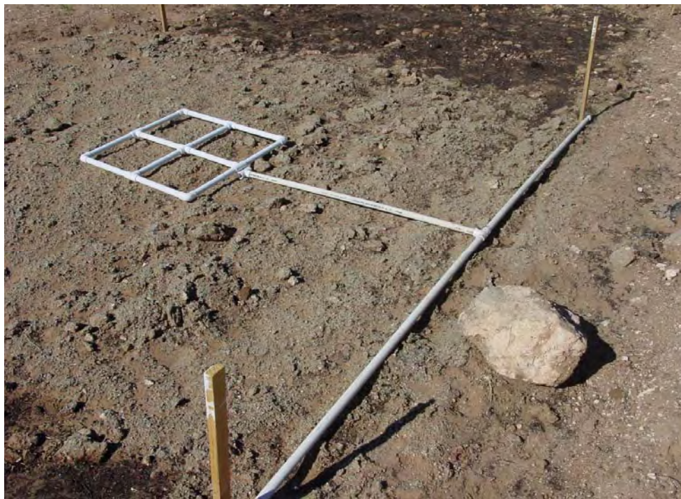
Figure 4.15 Designated Vegetation Quadrat on a Sub-Plot Treated With Cellulose Fiber Mulch at the Lubbock County Field Site
