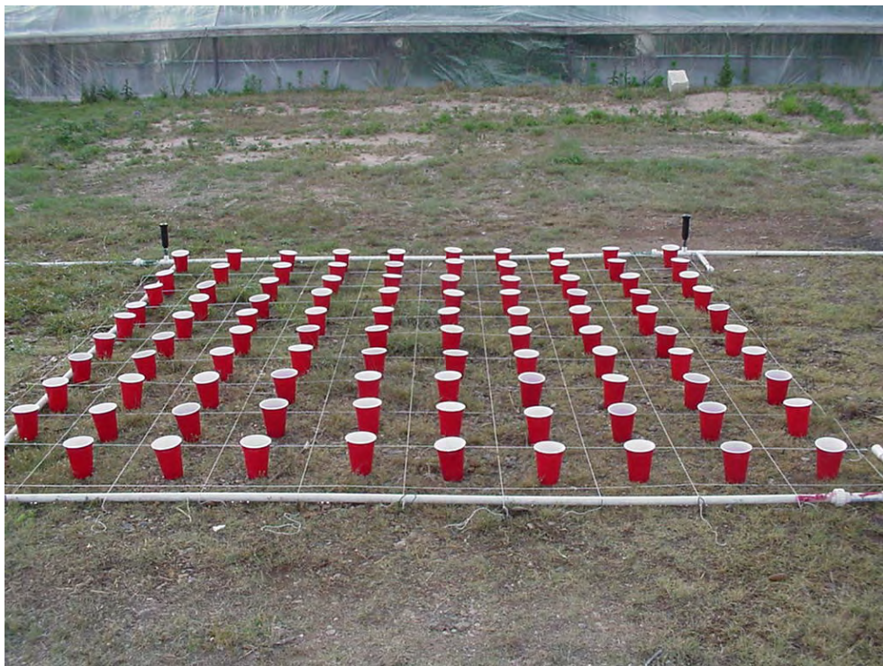
Figure 4.8 A 10 ft x 10 ft Irrigation System Test Section Used for Obtaining Christiansen's Uniformity Coefficient (UCC)
