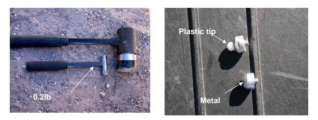
Figure 2 Instrumented Hammer with Interchangeable Metal/Plastic Tips
