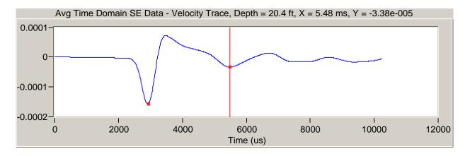
Figure 5 Typical Results Obtained from the Sonic Echo Test
