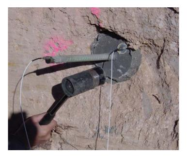
Figure 4 Hitting the Grout Column Head with 0.2-lb Hammer
