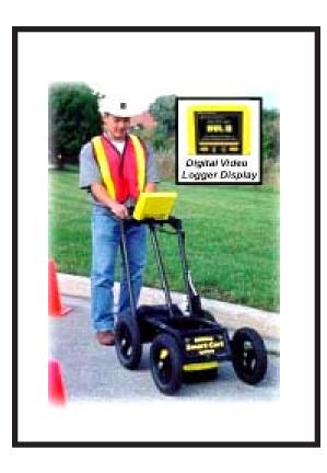
**Figure 3** Nogging Smart Cart from Sensors and Software Inc., in operating mode.
