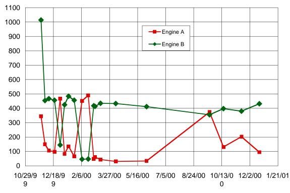
**Date Sample Taken** Figure A.6 Magnesium Concentration for Engine Oil Samples
