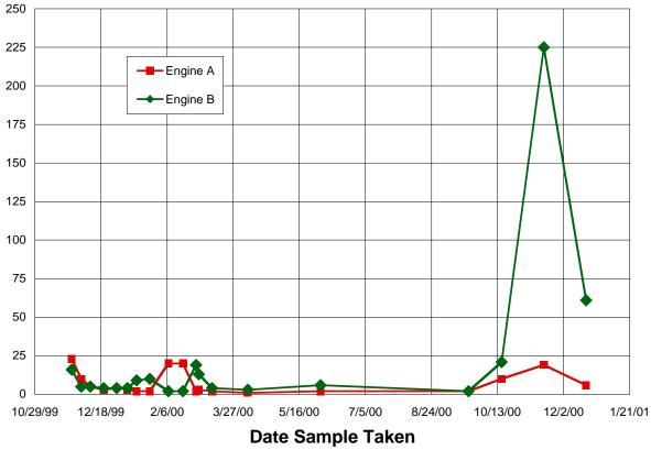
Figure A.9 Aluminum Concentration for Engine Oil Samples
