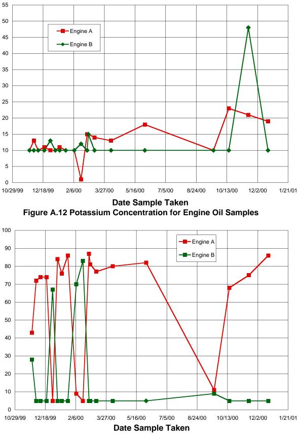
Figure A.13 Molybdenum Concentration for Engine Oil Samples
