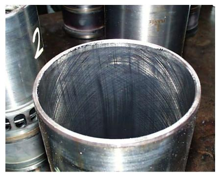
Figure B.6 Cylinder Liner
