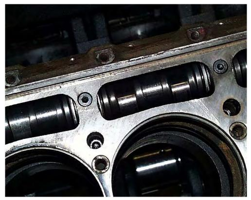
Figure B.2 Cylinder Deck Showing Cam and Cylinder Bore
