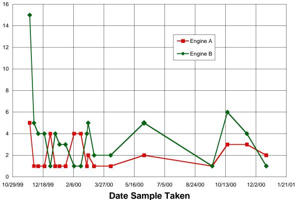
Figure A.7 Chromium Concentration for Engine Oil Samples
