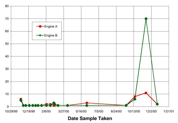
Figure A.8 Lead Concentration for Engine Oil Samples
