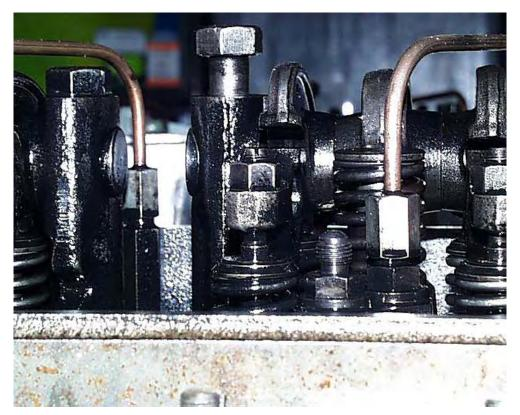
Figure B.5 Top of Cylinder Head
