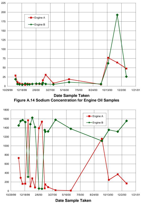
Figure A.15 Phosphorus Concentration for Engine Oil Samples
