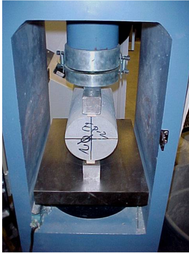
Fig. 2.26 Split cylinder test set-up
