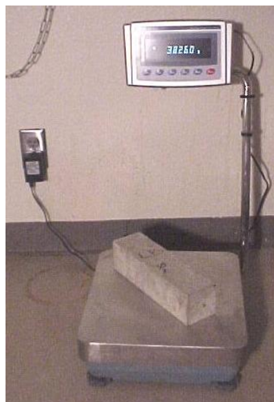
Figure 2.20 Measuring Weight of Shrinkage Specimen
