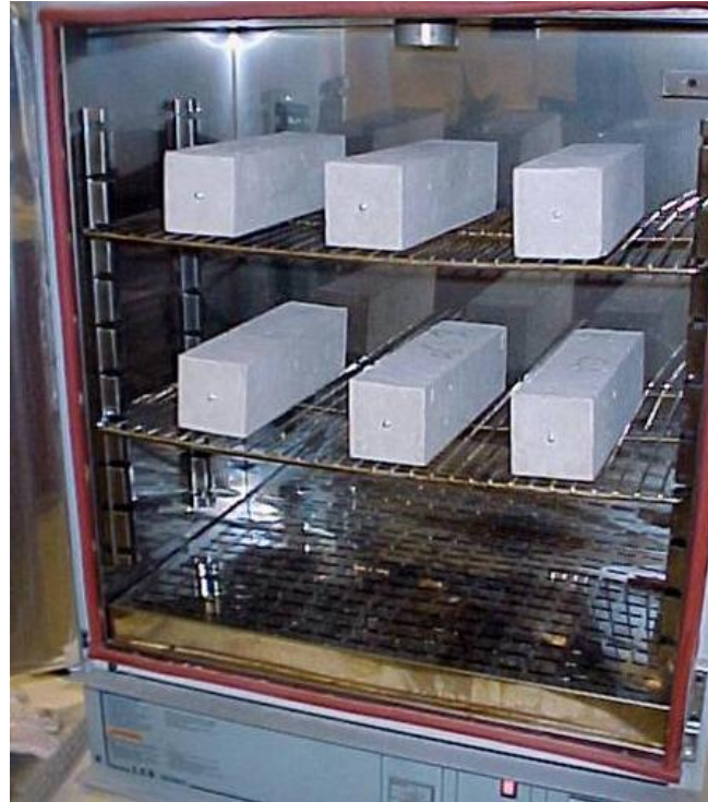
Figure 2.21 Specimens placed in the oven for drying at 110 0 C
