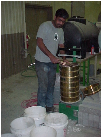
Figure 2.5 Coarse Aggregate being Sieved
