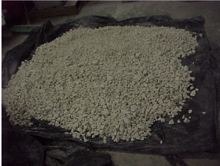
Figure 2.4 Coarse Aggregate being Air-Dried.
