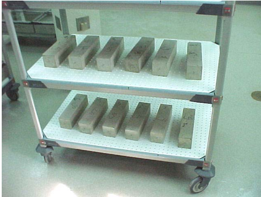
Figure 2.17 Shrinkage specimens being dried in a controlled environment
