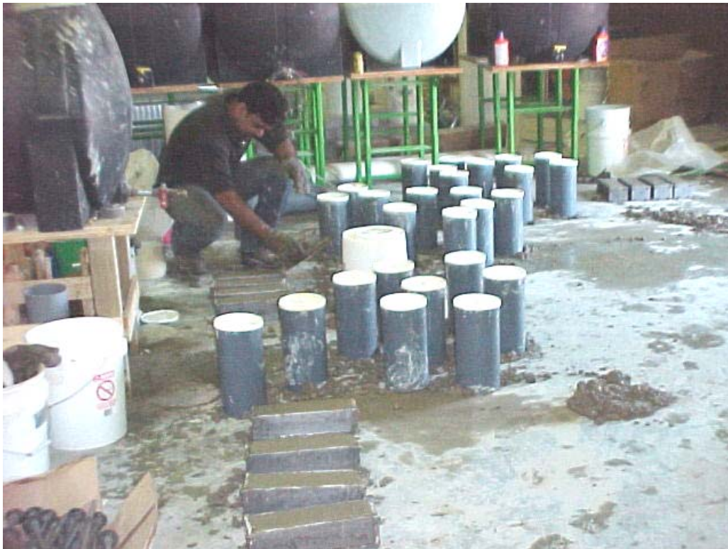
Fig. 2.22 Finishing Specimens Cast for El Paso District Mix
