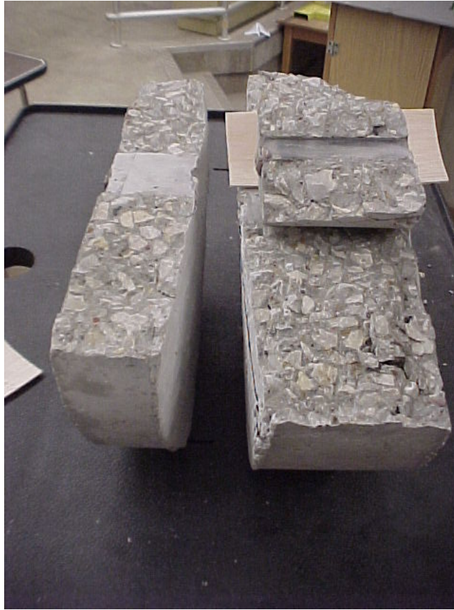
Figure 3.28 Differences in Hydrated Products Shown on Fractured Surfaces.
