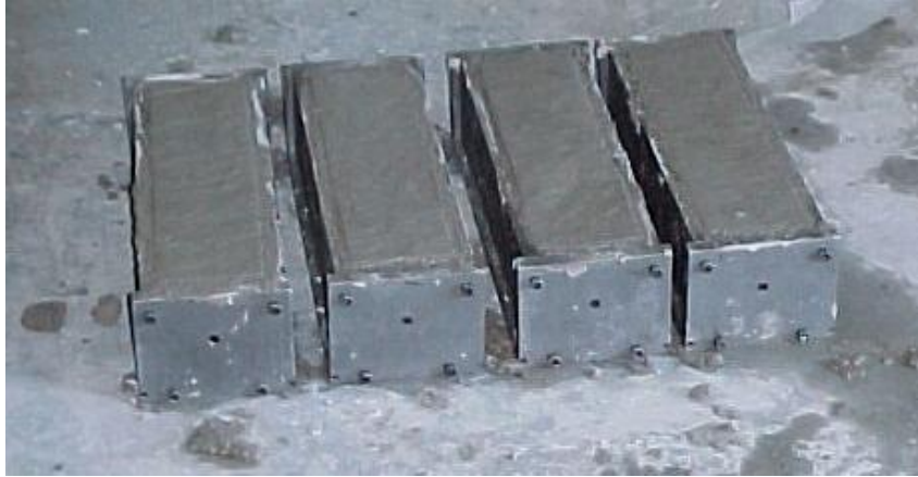
Figure 2.16 Shrinkage specimens in molds immediately after finishing
