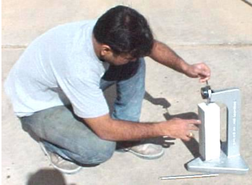
Figure 2.19 Taking Length Comparator Reading of the specimen
