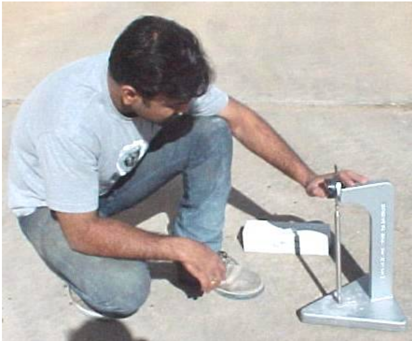
Figure 2.18 Setting Length Comparator Reading to zero for the reference bar
