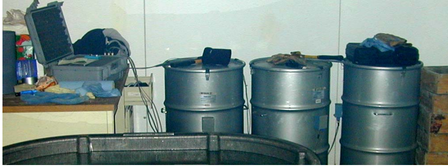
Figure 2.17 Calorimeter Drums and Data Logger
