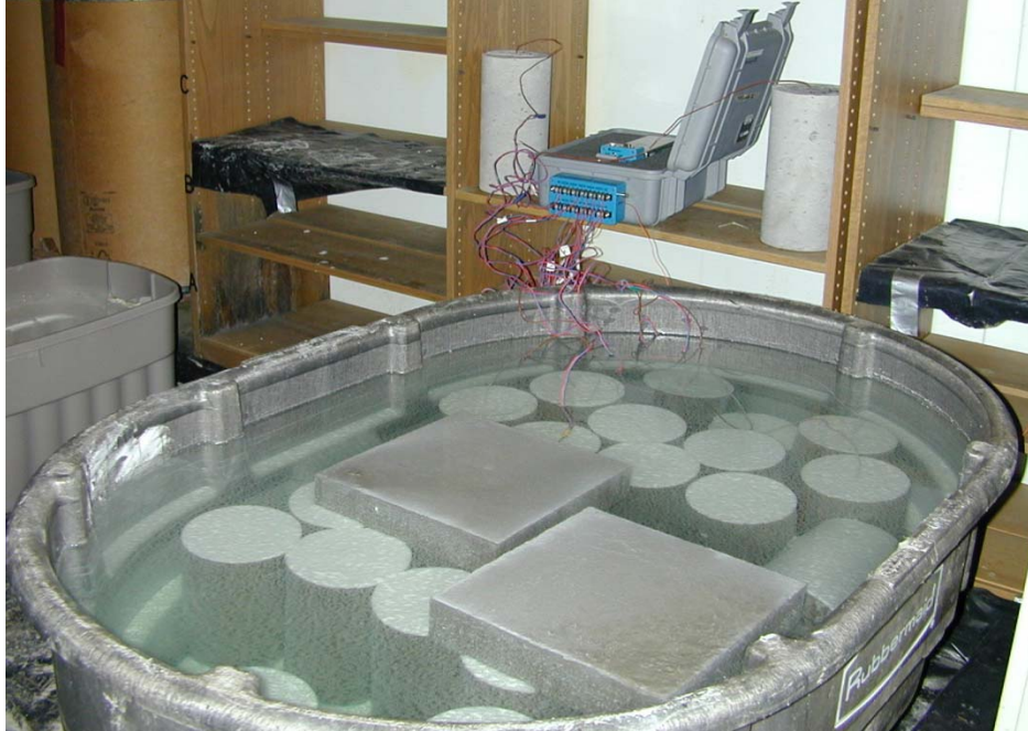
Figure 2.16 Lab Cylinders with Embedded Thermocouples in Lime Bath
