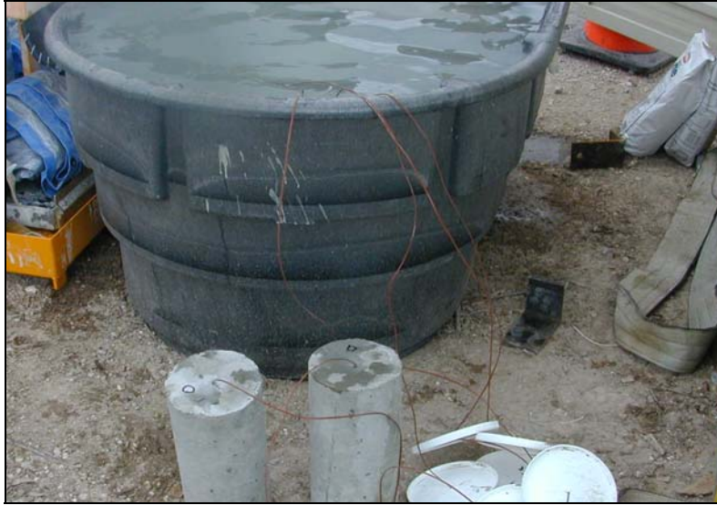
Figure 2.14 Lime Bath and Cylinders with Embedded Thermocouples
