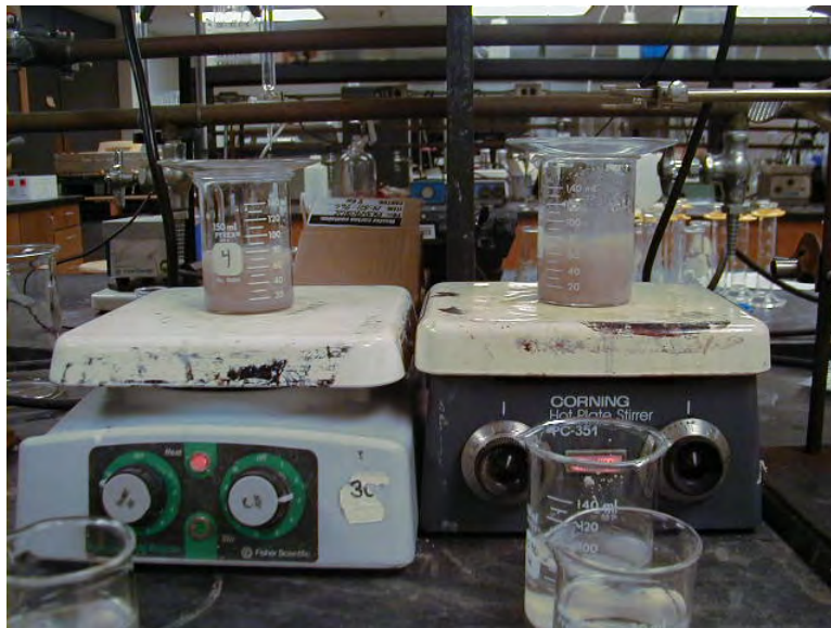
Figure 4.9 Boiling the Specimen for Five Minutes
