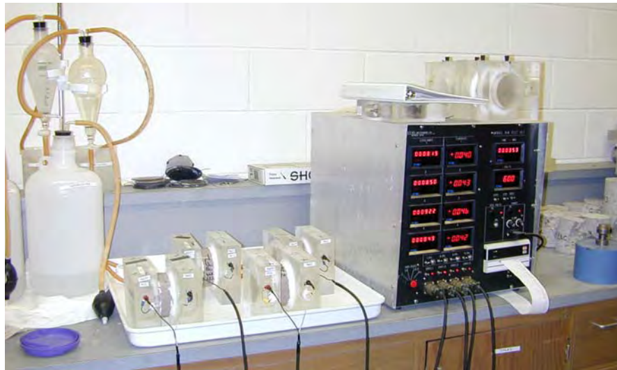
Figure 3.1 RCPT Test Setup
