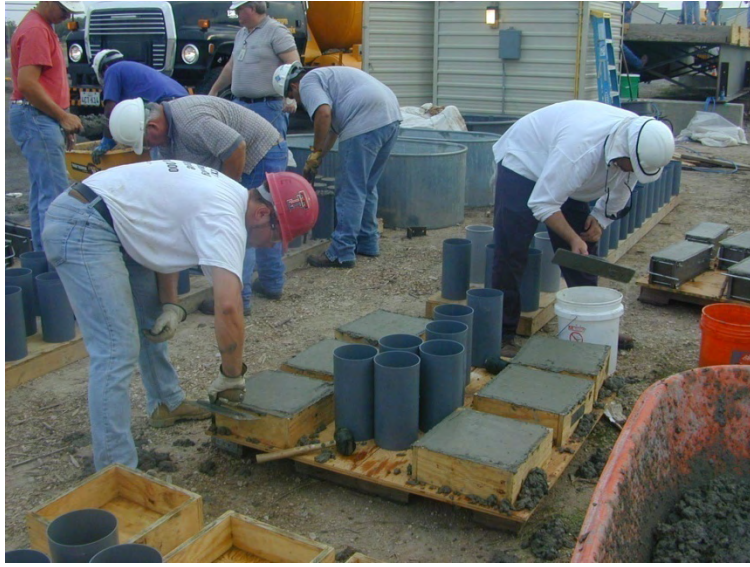
Figure 1.2 Casting of the 12"×12" Specimens
