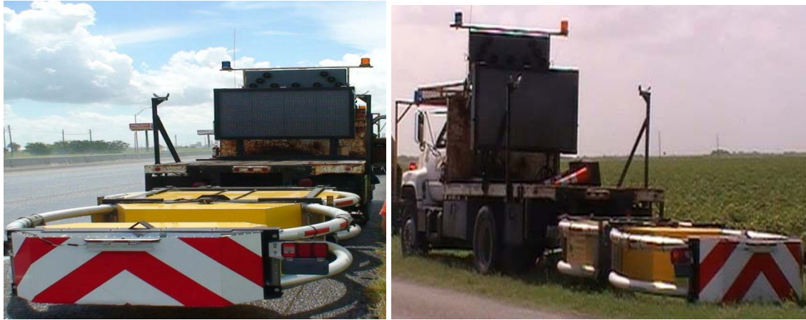
Figure 20. Rear and Side View of TMCMS Used for Field Evaluations.
