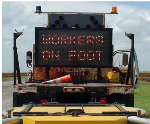
Figure 21. CMS Display Board Installed on TMCMS.
