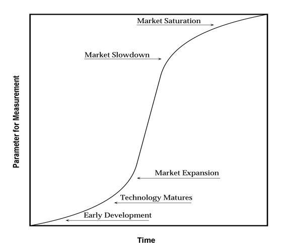
**Figure 1.5** Various stages in the diffusion of new technology in the market place. This is the classic S-shaped logistic function (as represented in the log-function of equation 3) plotted on a linear scale. A log transform will give a straight line with a slope equal to alpha  $(\alpha)$  and the intercept equal to beta  $(\beta)$ ,
