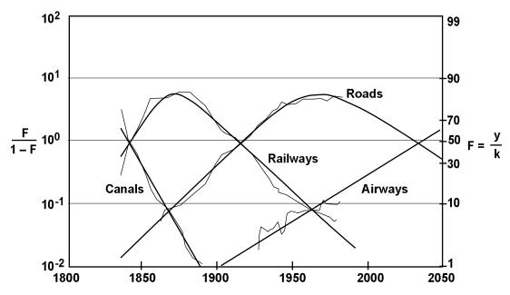
**Figure 1.4** Substitution of transport infrastructures in the U.S., shares in length, logistic transformation. Actual data are thin lines, estimated logistic curves are thick lines. [Adapted from: Nakicenovic (1988).]
