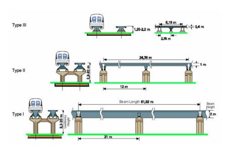
Figure 5.5 The three main types of guideways,
