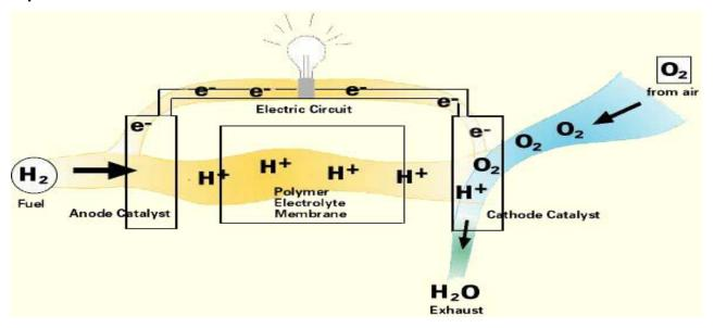
**Figure 4.1** Working of a Fuel Cell, (Data source: <a href="http://www.fuelcells.org/whatis.htm">http://www.fuelcells.org/whatis.htm</a>)
