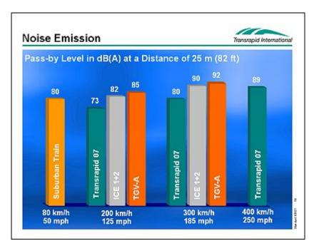
**Figure 5.12** Comparison between noise produced by Transrapid and high speed trains, (Data source: Transrapid International)
