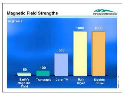
**Figure 5.13** Comparison between magnetic field strength of Transrapid and that of household appliances, (Data source: Transrapid International)
