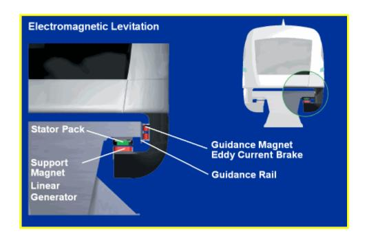
**Figure 3.6** Mechanism of Magnets (Data source: www.transrapid.de/en/index/html)
