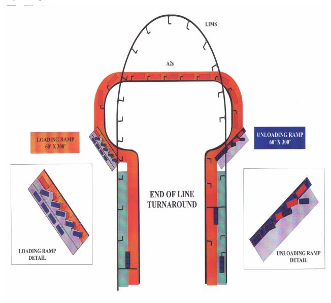
Figure 3.17: A schematic explaining End of Line Turnaround for A2
