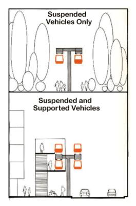
Figure 3.12 Two types of PRT System
