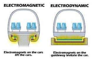
**Figure 5.3** The two basic types of levitations in Maglev, (Data source: The Science of Maglev)
