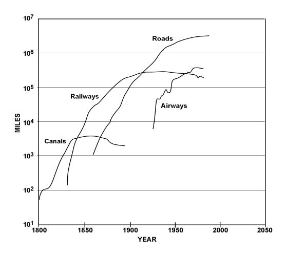
**Figure 1.1** Length of canals, railroads, surfaced roads, and federal airways in the U.S. [Adapted from: Grübler & Nakicenovic (1991).]
