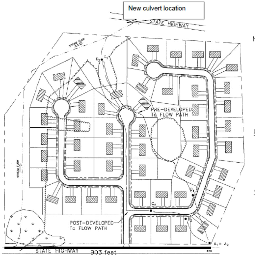
Figure 4.1: Subdivision X Drainage to a Highway Culvert
