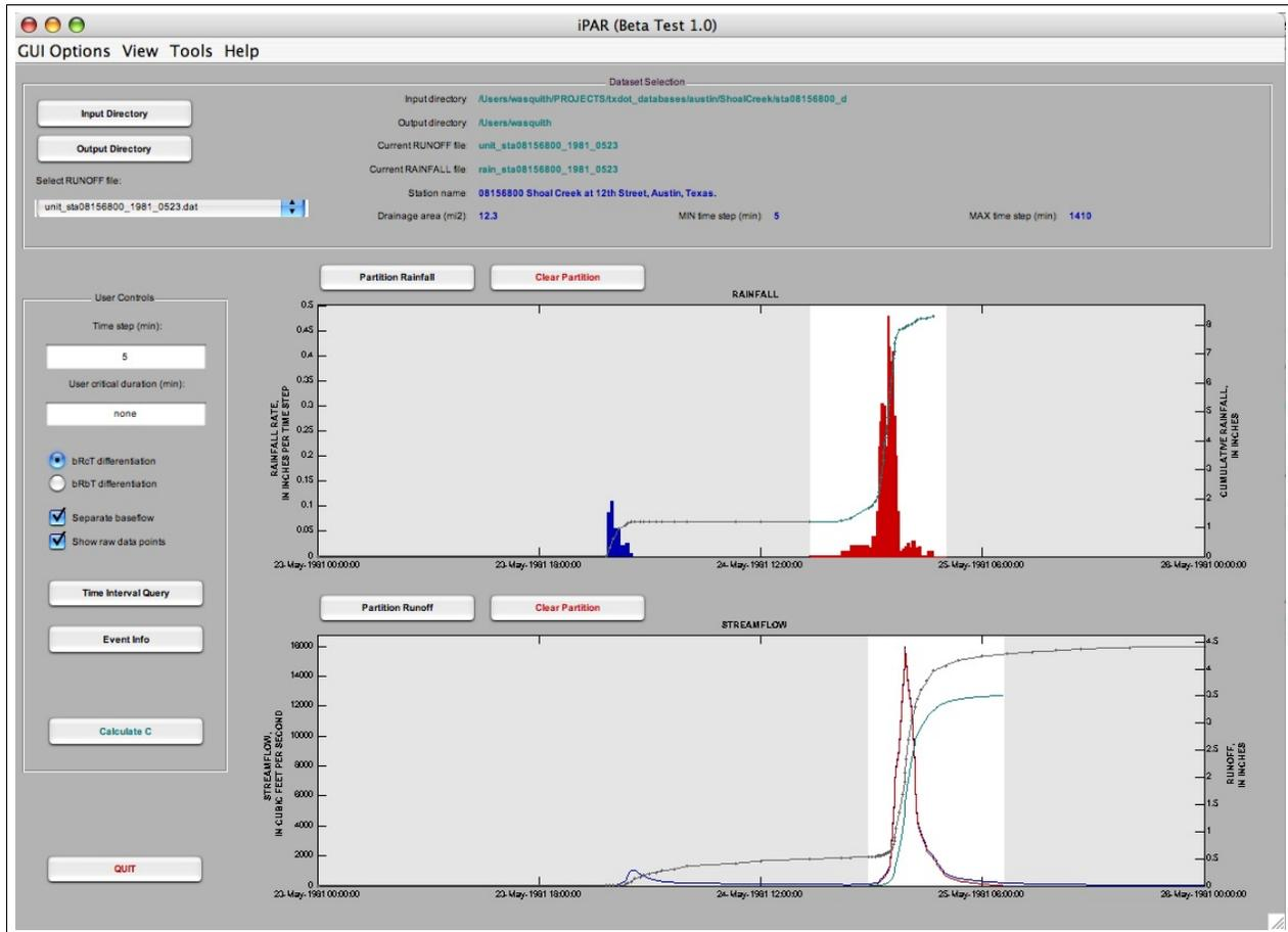
Figure C.2: Screenshot of custom-built *iPAR* program used to parse a historically significant flood event at U.S. Geological Survey streamflow-gaging station 08156800 Shoal Creek at 12th Street, Austin, Texas, May 24, 1981, which has a drainage area of about 12.3 square miles. The top plot shows the incremental rainfall and the bottom plot shows the resultant runoff hydrograph.
