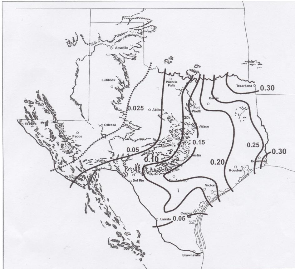
Figure A.4: Runoff Coefficients for Texas from Ward (2005). **Warning:** This figure is not appropriate for drainage design using the rational method at a small spatial or temporal scale — it [the figure] is constructed from basin-scale water budget studies.
