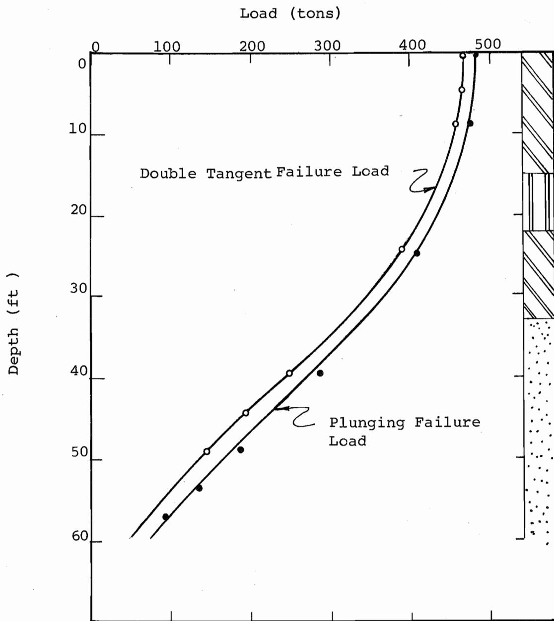
Figure 5.4. Load Distribution Curves,
