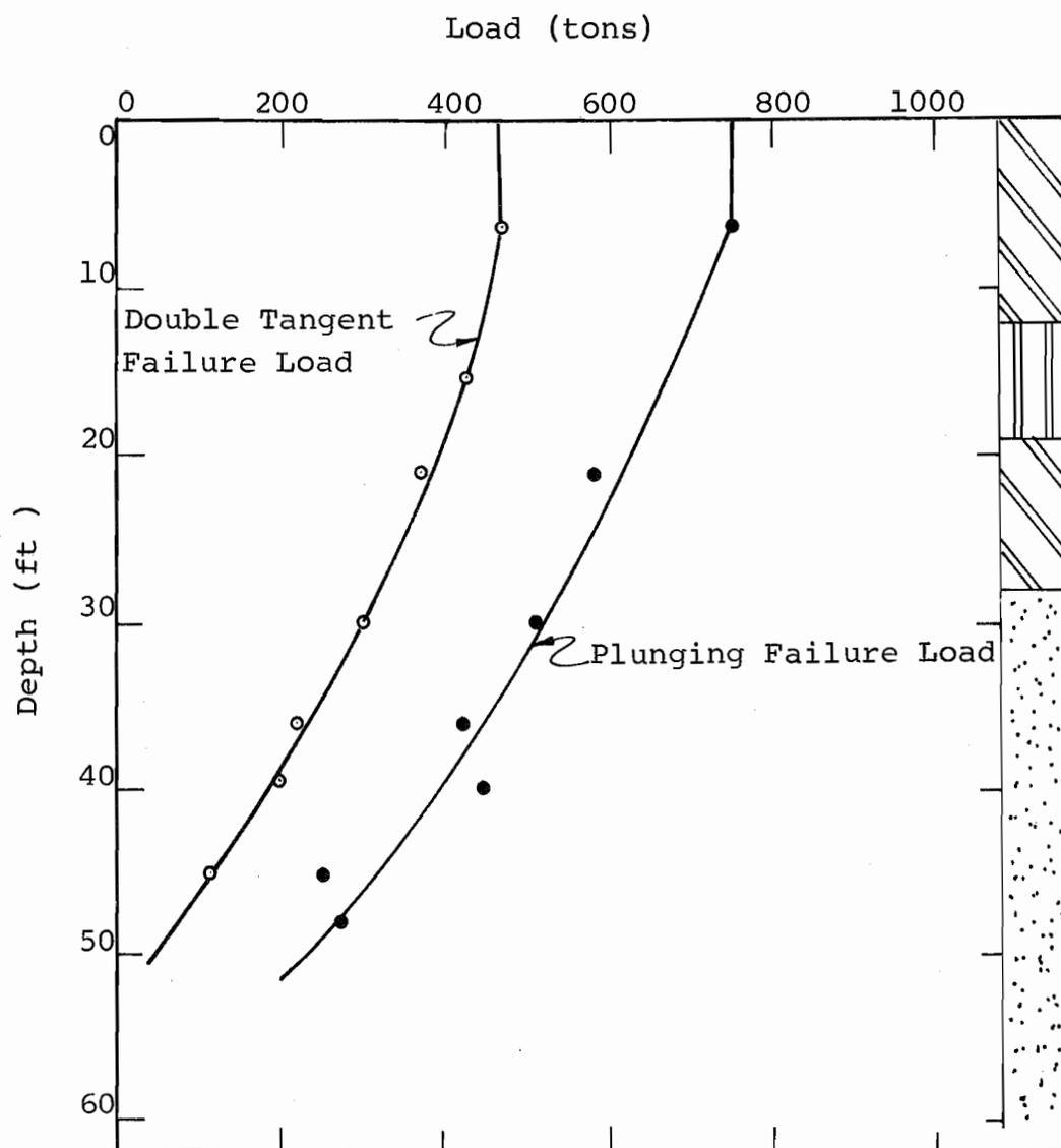
Figure 5.6. Load Distribution Curves, Shaft BB, Test No. 1
