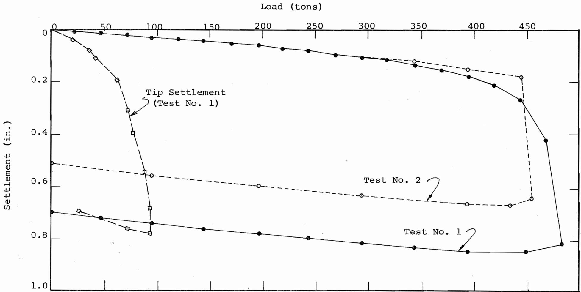
Figure 5.1. Load-Settlement Curves, Shaft G 1
