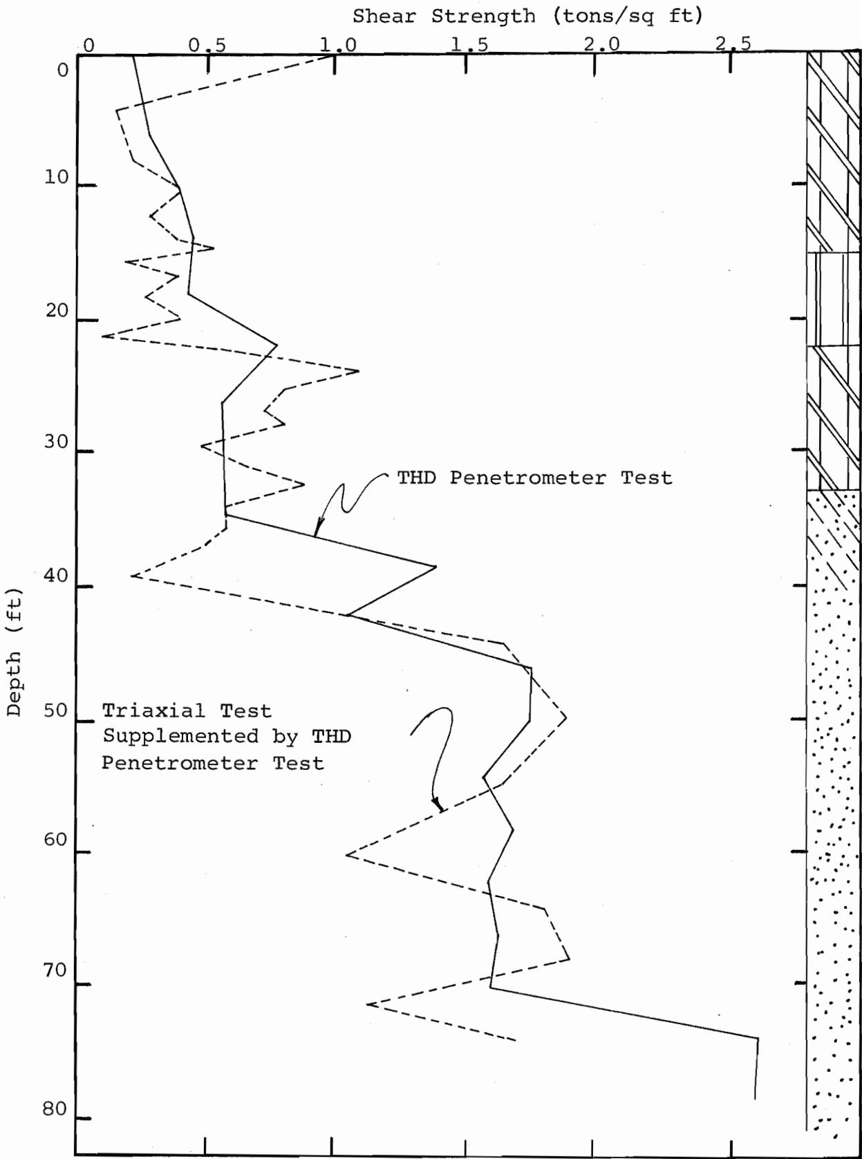
Figure 2.2. Shear Strength Profile for Site G 1
