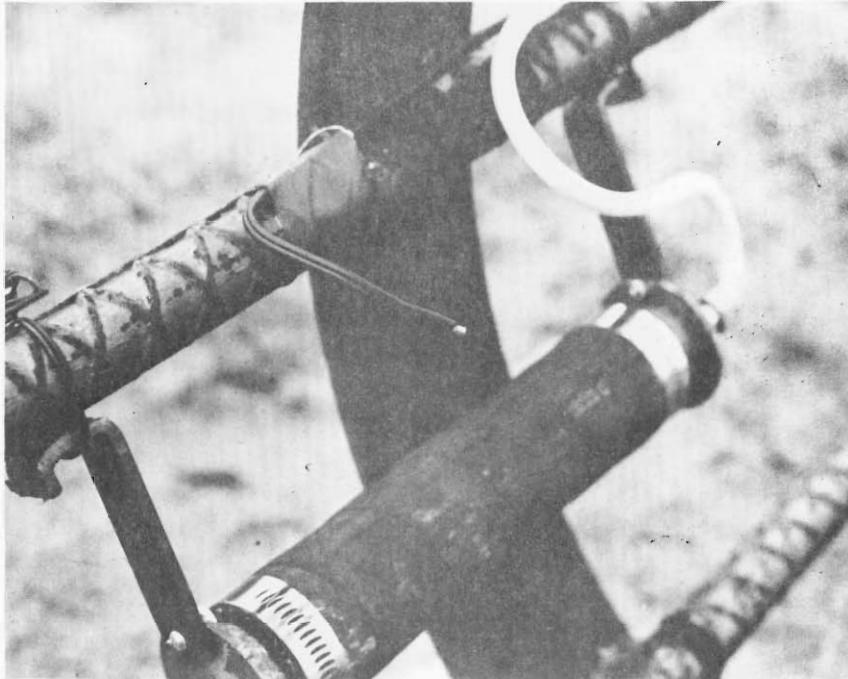
Figure 3.6. Mustran Cell Attached to Reinforcing Steel
