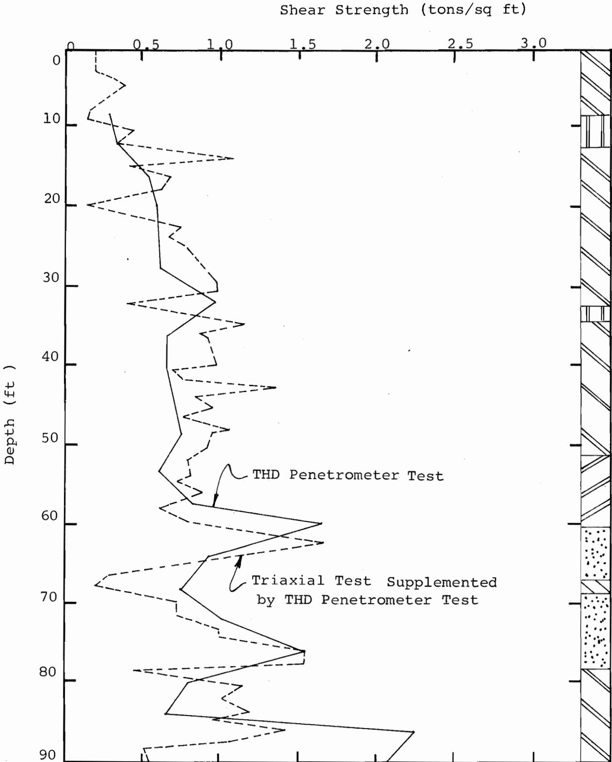
Figure 2.3. Shear Strength Profile for Site G 2
