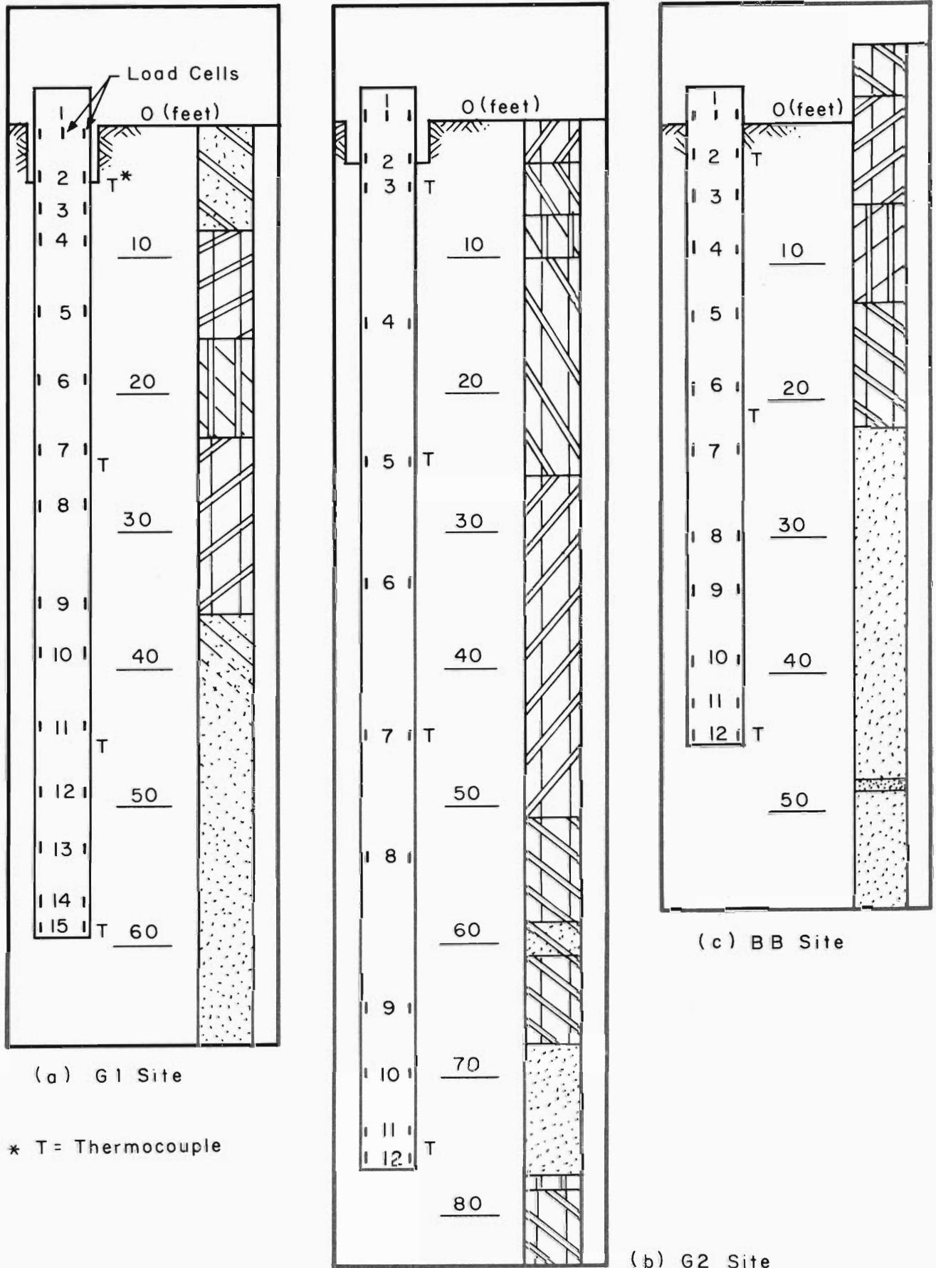
Figure 3.5. Soil Profiles and Location of Shaft Instrumentation
