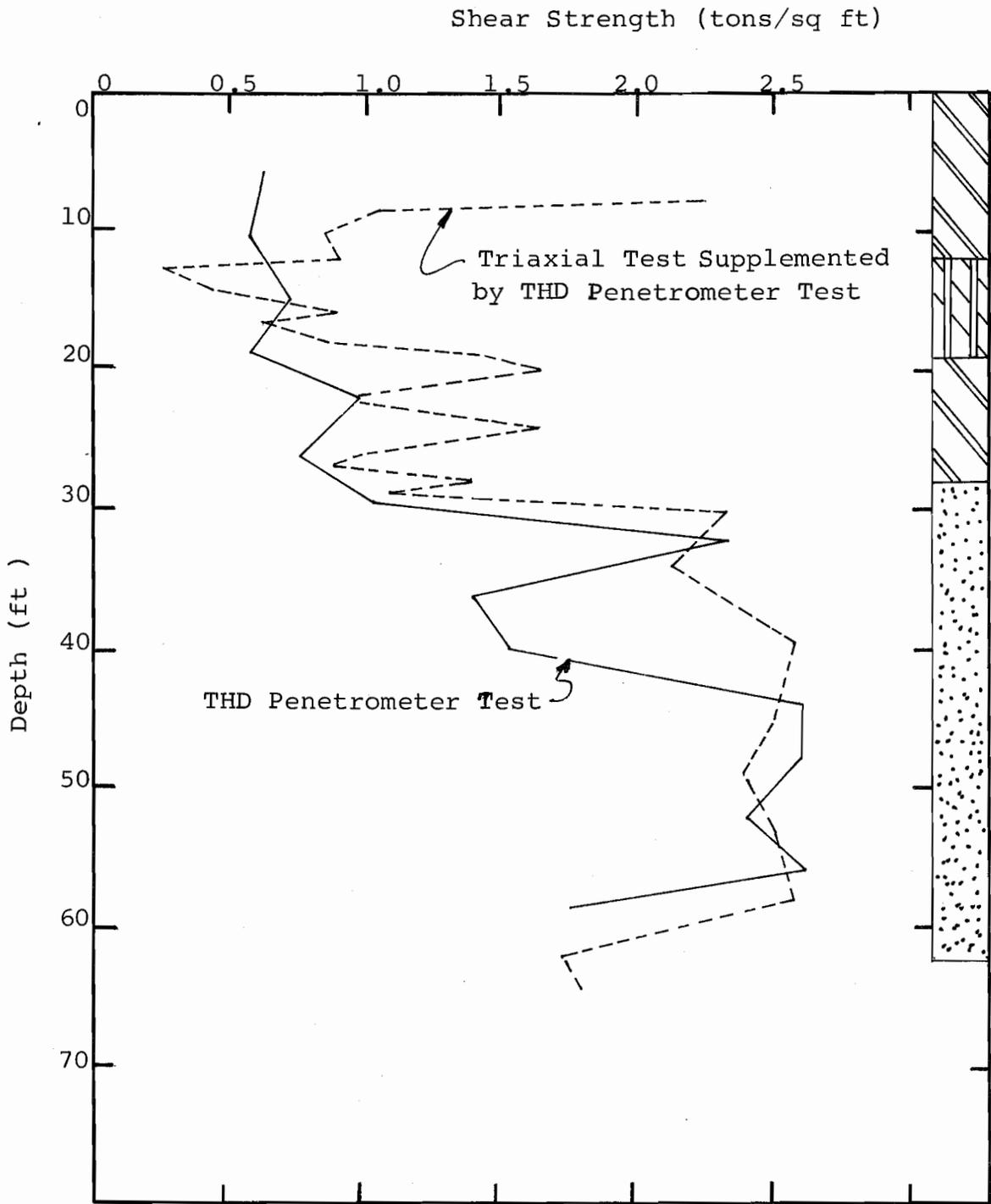
Figure 2.4. Shear Strength Profile for Site BB
