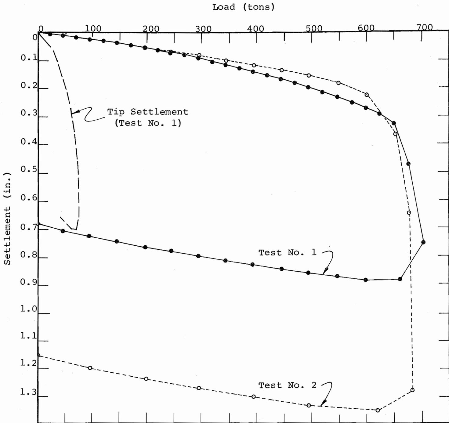
Figure 5.2. Load-Settlement Curves, Shaft G 2
