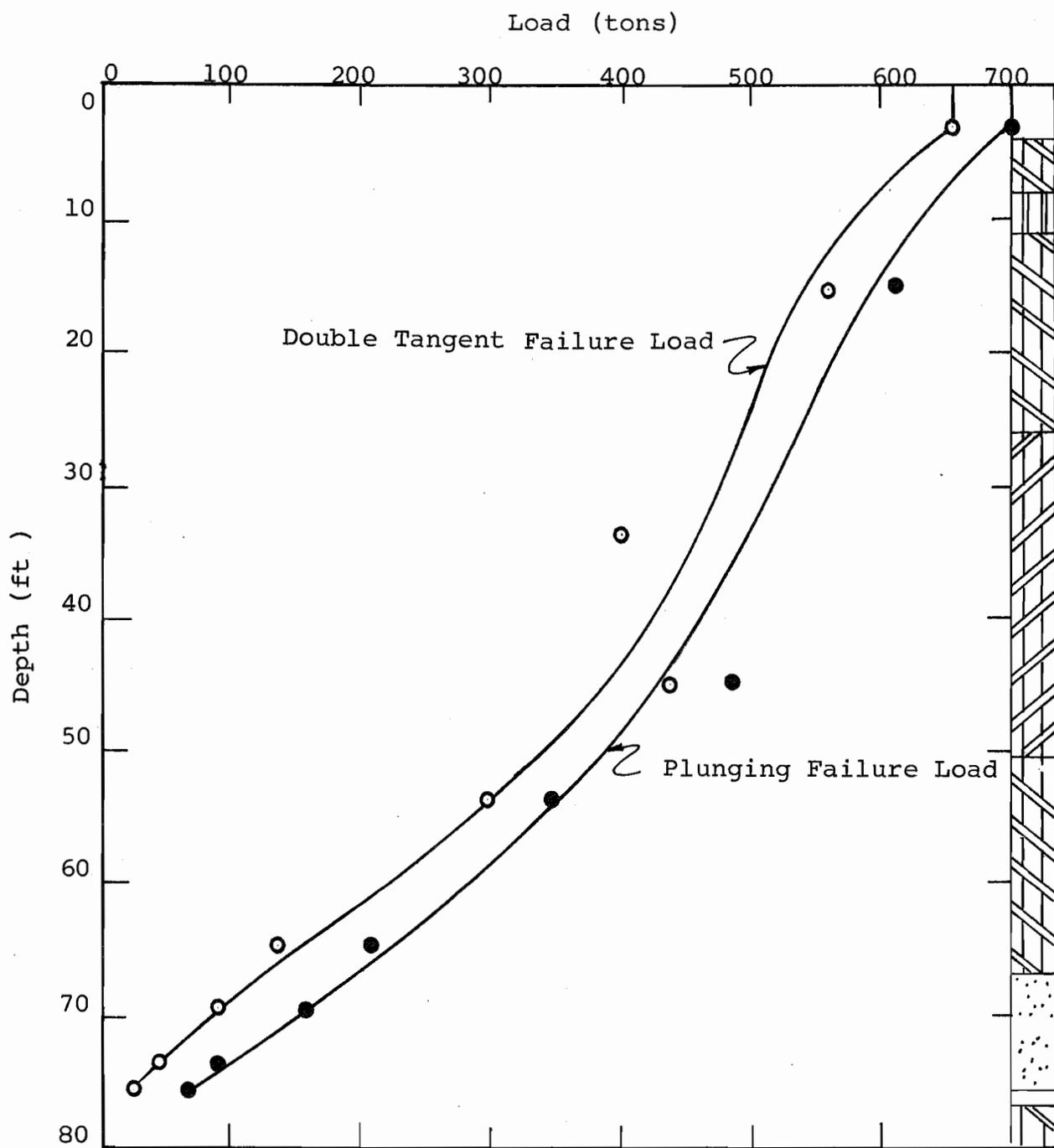
Figure 5.5. Load Distribution Curves, Shaft G 2, Test No. 1
