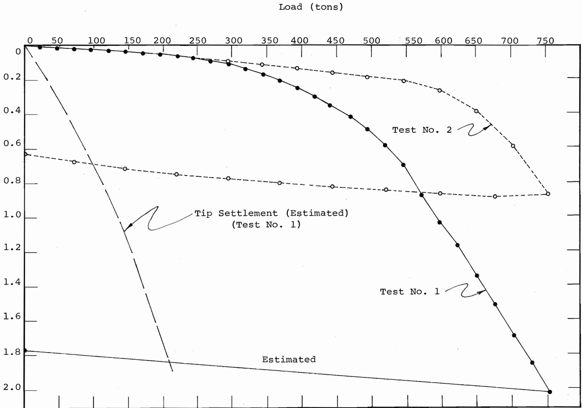
Figure 5.3. Load-Settlement Curves, Shaft BB
