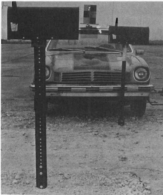
Figure 20. Mailbox Supports Before Tests 3-1 and 3-2.
