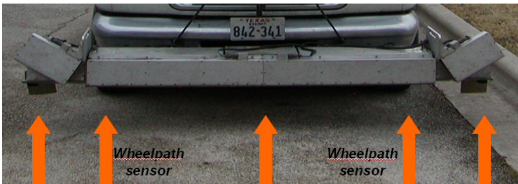
Figure 1. TxDOT Five-Point Sensor Rut System.
