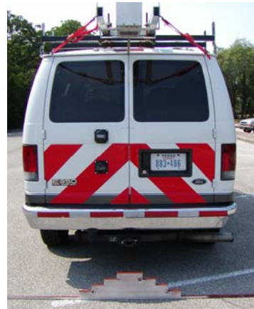
b) Laser triangulation calibration
