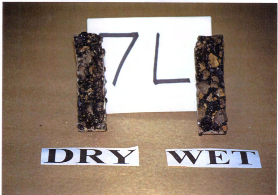
Figure 1A. Cores from Lufkin-7 Section. Visual stripping ratings are 2.5 and 1.8 for Dry and Moisture Conditioned Specimens, respectively.
