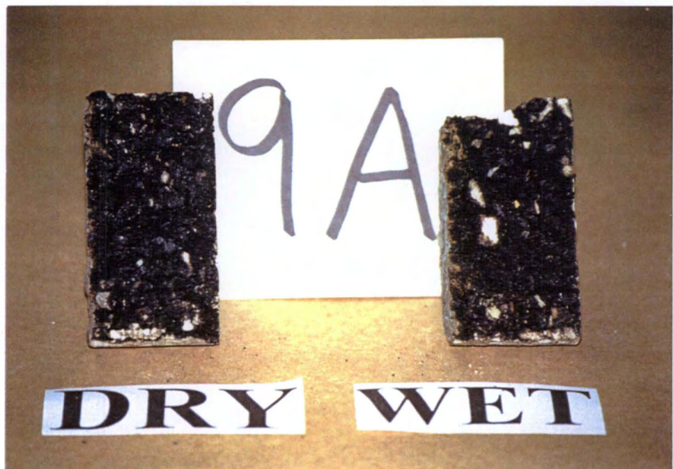
Figure 1B. Core from Atlanta-16 Section. Visual stripping ratings is 4.9 for both Dry and Moisture Conditioned Specimens.
