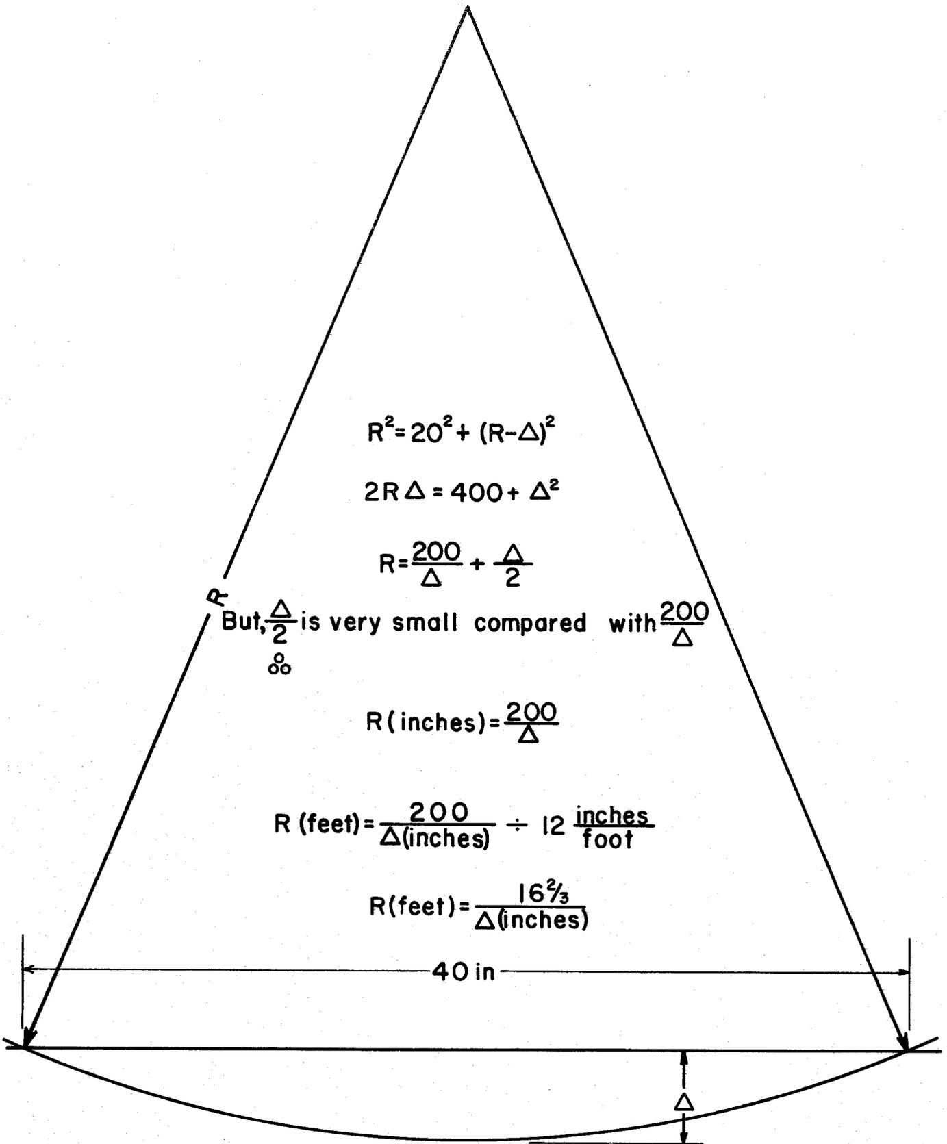
DERIVATION OF CIRCULAR RADIUS OF CURVATURE FROM BASIN BEAM
