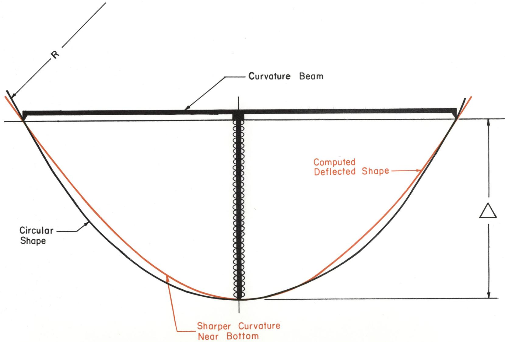
COMPARISON OF COMPUTED DEFLECTED SHAPE AND CIRCULAR SHAPE OF LOADED PAVEMENT
