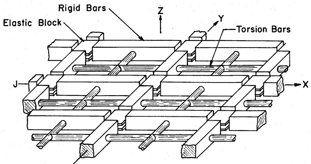
FINITE ELEMENT MODEL OF A PLATE OR SLAB
