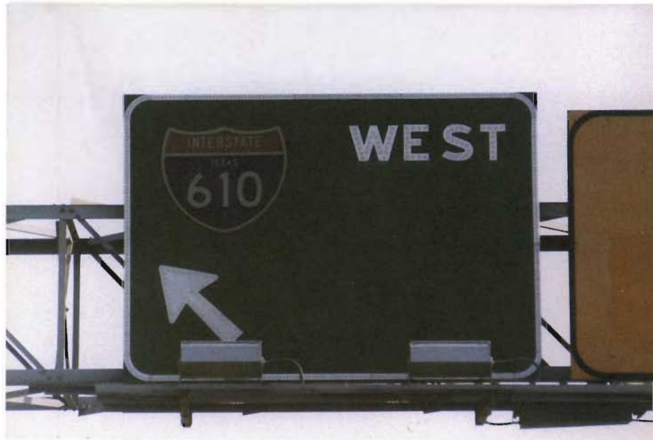
Sign Panel Refurbished Using Acrylic Cured Aliphatic Urethane after 10 Years Field Service
