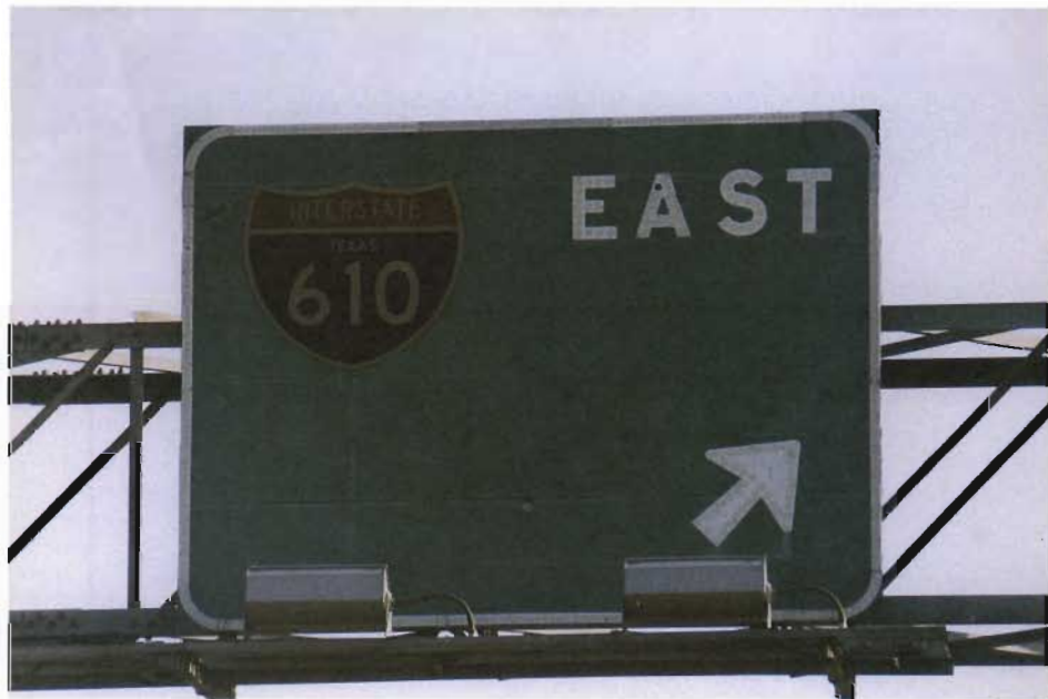
Sign Refurbished with GES-2C Sign Enamel after 10 Years Field Service
