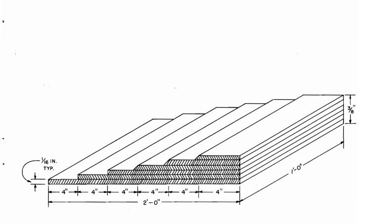
Figure A-I CALIBRATION SPECIMEN I
