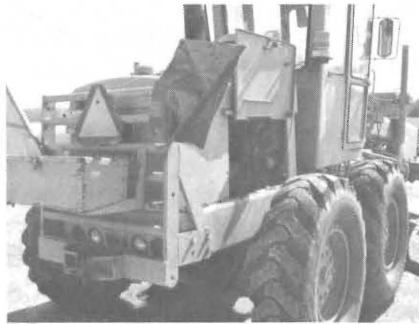
FIGURE 6 The framework protecting the fuel tank.
