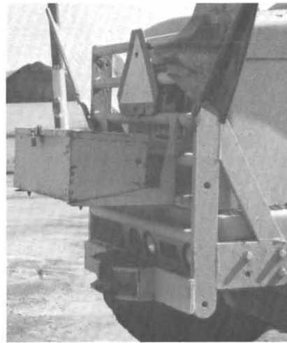
FIGURE 7 Note toolbox and hitch mounted on the framework.
